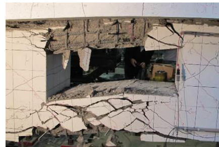
Fig. 5a & b: – Crack patterns in specimen S1 at drift ratio 4.5% (a, left) and photograph of opening region cracks and damage at drift ratio 4.5% (b, right)
