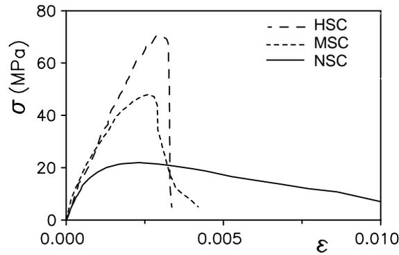
**Figure 1: Results in compression for plain concrete at different strength**
