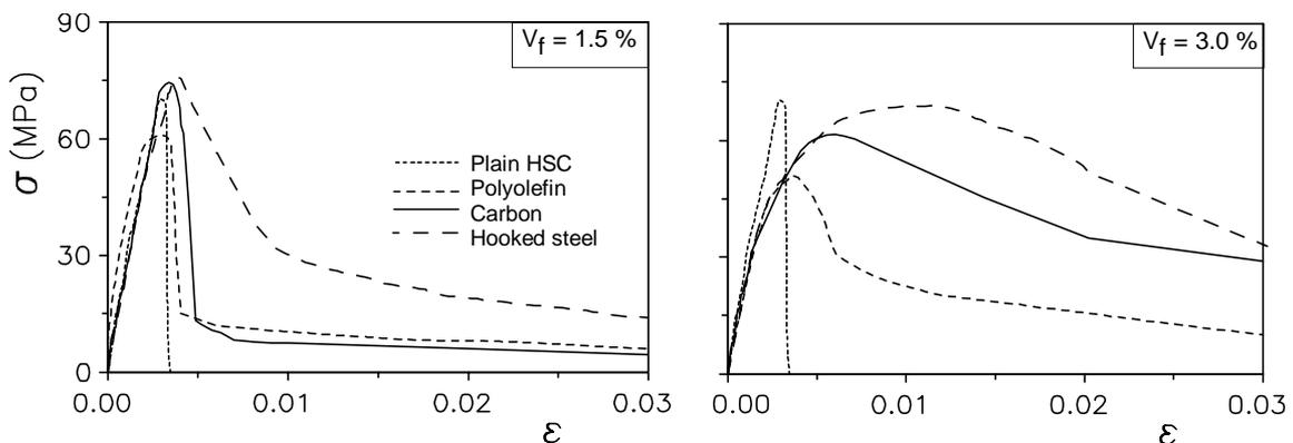
**Figure 3: Stress-strain curves of fibre reinforced concrete at different types and percentages**
