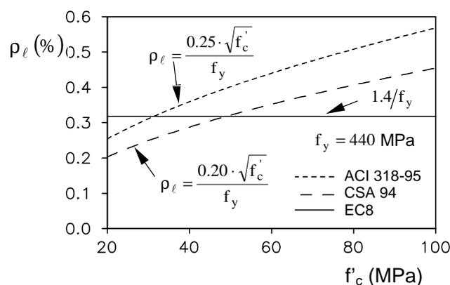
Figure 7: Minimum flexural reinforcement
