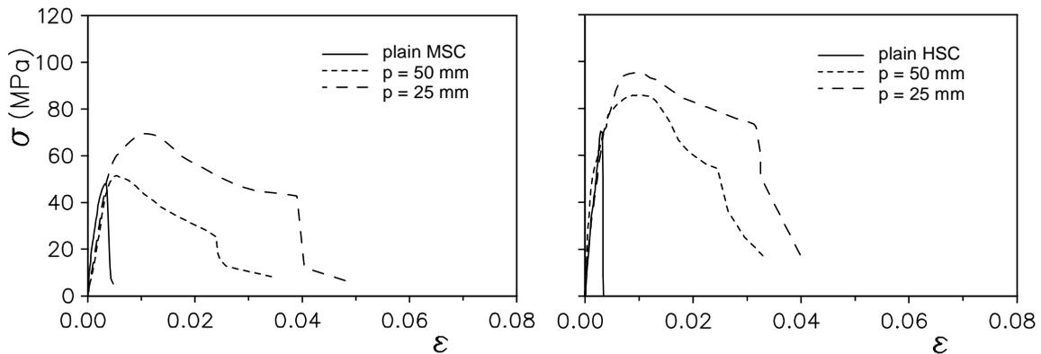
**Figure 2: Stress-strain curves of plain concrete ( $V_f = 0$ ) with steel spirals**
