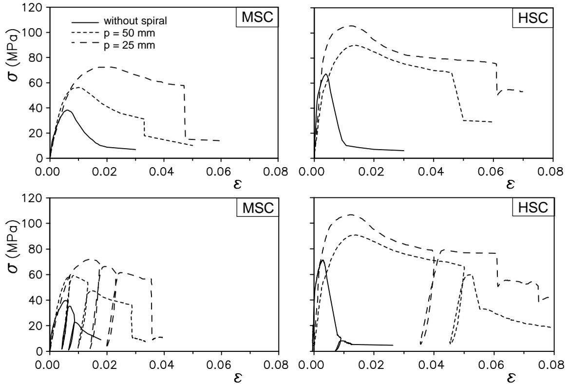
**Figure 4: Monotonic and cyclic  $\sigma$ - $\epsilon$  curves of carbon fibre ( $V_f = 2\%$ ) reinforced concrete with steel spirals**
