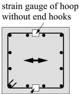
strain gauge of hoop with 135 degree hooks
