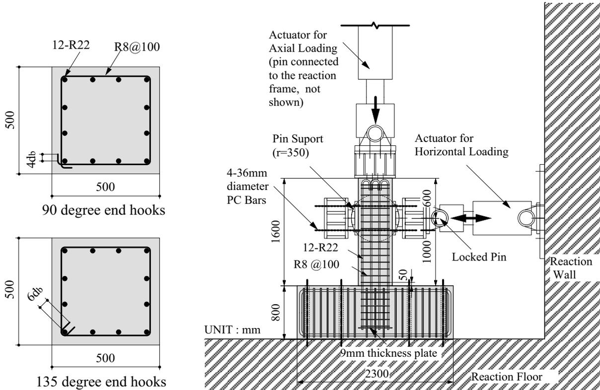
Figure 1: Column sections and Unit 1 as tested
