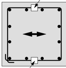
strain gauge of hoop with 90 degree hooks
