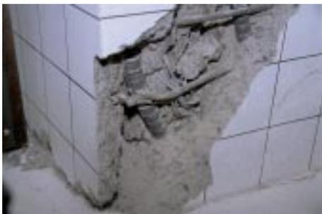
(e) 90 degree end hooks after testing
