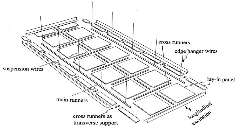
Fig.2 Test Sample Configuration
