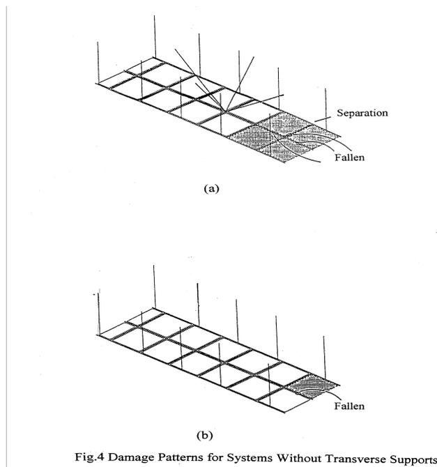
Fig.4 Damage Patterns for Systems Without Transverse Supports
