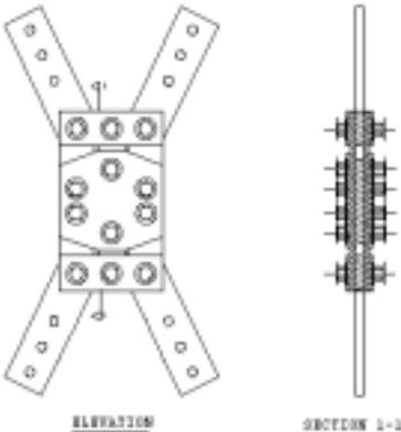
**Figure 2: Pall friction damper**
