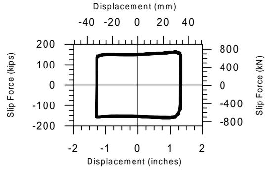
**Figure 4: Hysteretic loop of prototype friction damper**
