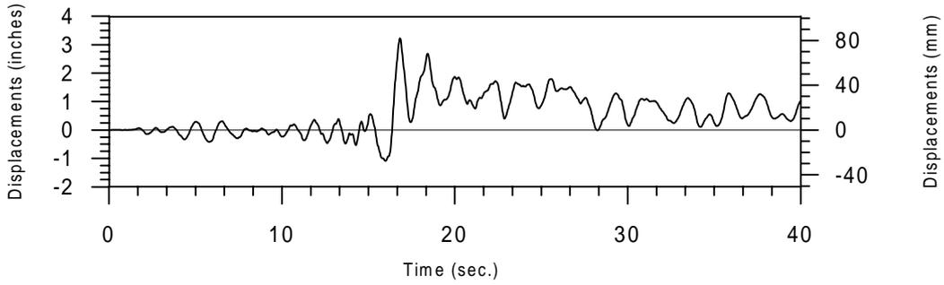
**Figure 5: Horizontal displacement at tank level - Z direction - BSE-1 Landers earthquake**
