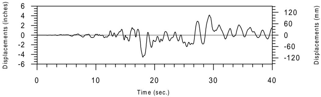
**Figure 6: Horizontal displacement at tank level - X direction - BSE-2 Landers earthquake**
