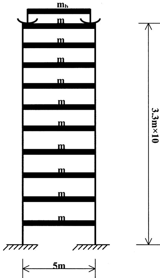
Figure 2. Example shear structure with TMD at top.
