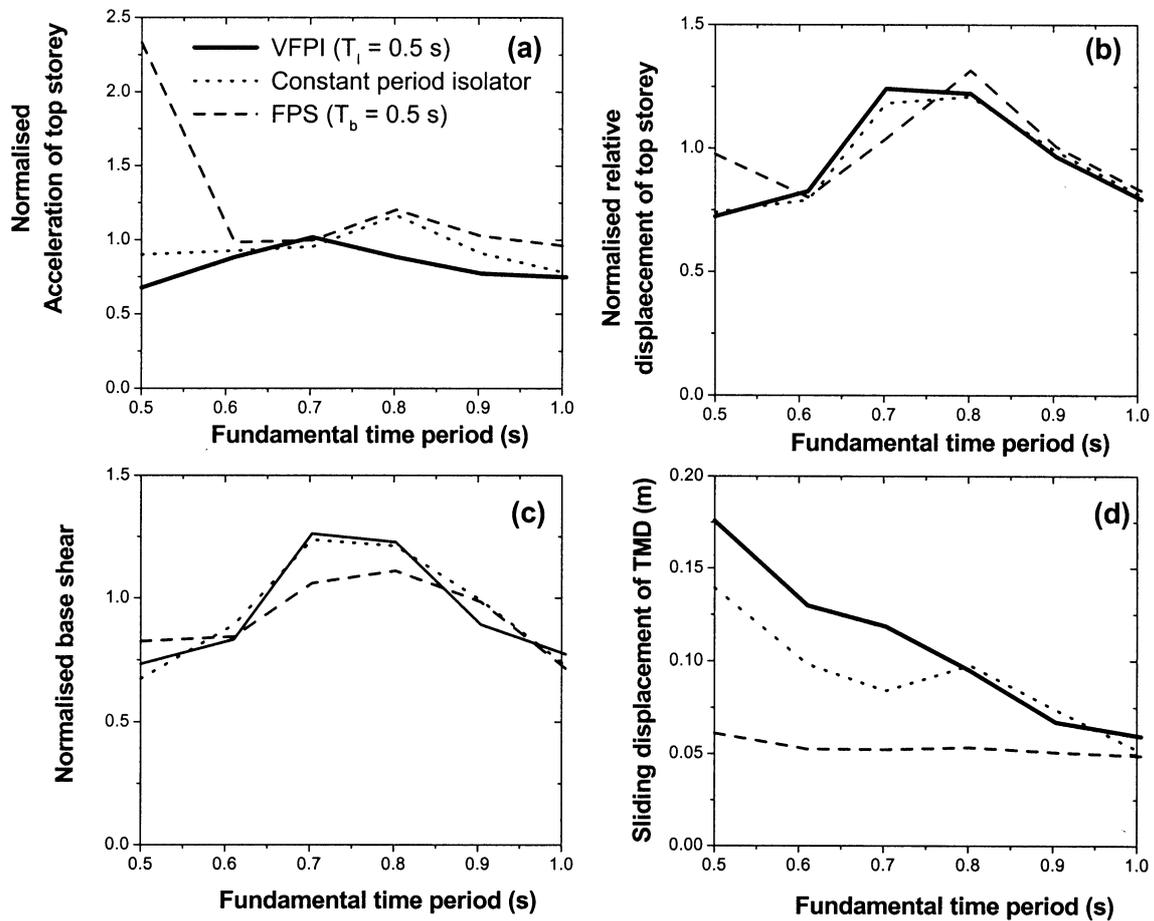
Figure 4. Structural response of example building with TMD subjected to El Centro 1940(NS) ground motion ( $T_1 = 0.5$ s, FVF = 1.0,  $\mu = 0.02$ ,  $\xi = 5\%$ ).
