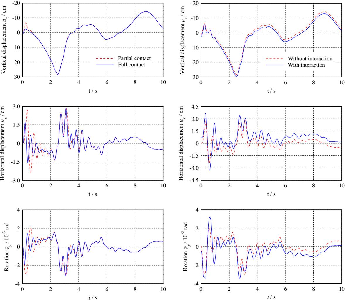
a) Influence of partial contact (without structure B)      b) Influence of the adjacent structure B (partial contact)
