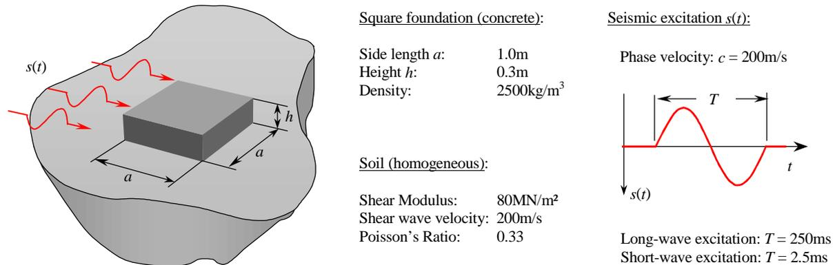
**Figure 4 System under investigation and time history of the seismic excitation**
