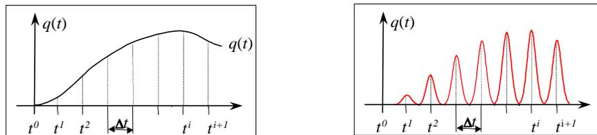
**Figure 3** Representation of the continuous contact stresses by a sequence of modified impulses
