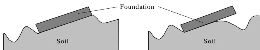
**Figure 1** Conditions of contact. Left: full contact, right: partial contact
