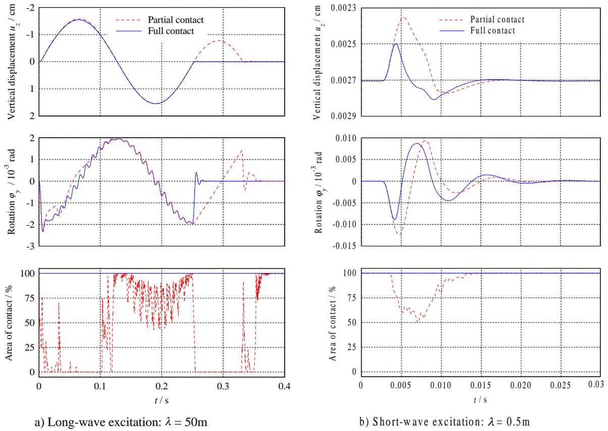
**Figure 5** Square foundation subjected to a seismic excitation: Influence of full and partial contact
