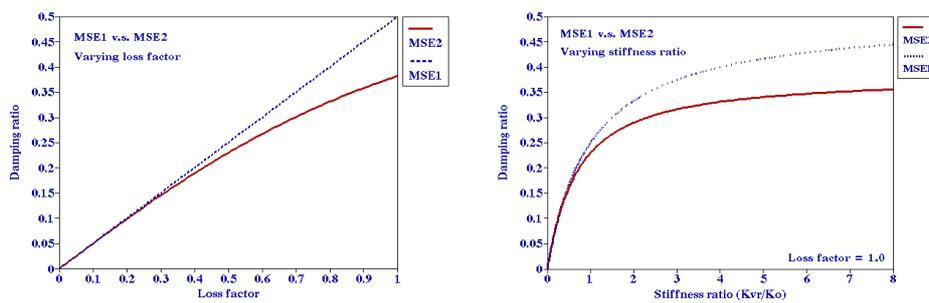
**Figure 1(left) and 2(right): Comparison of predicted damping ratios**
