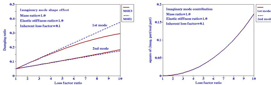
**Figure 3a (left): Effect of imaginary mode shape on predicted damping ratio**
