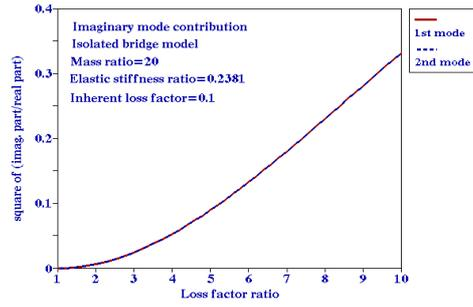
**Figure 5a (left): Predicted damping ratios for a typical isolated bridge model**
