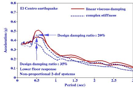
**Figure 7a (left): Acceleration response spectra of the non-proportional systems (top floor)**
