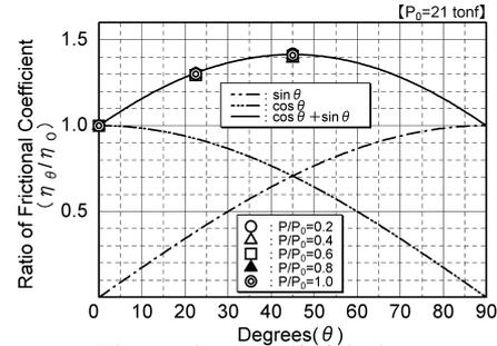
Figure-8: angle & friction
