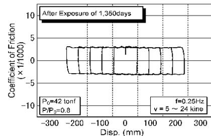
(b) Coefficient of Friction After Exposure
