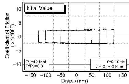
(a) Coefficient of Friction Before Exposure
