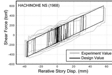
Figure-18: disp.-load curve
