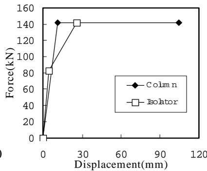
**Figure 4. Force-Displacement Relation of the Seismic Isolator and the Column Specimen**
