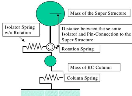
**Figure 10. Schematic Image of the Tested Bridge Model**
