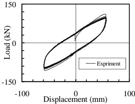
**Figure 3. Load-Displacement Test Result of the Seismic Isolator**
