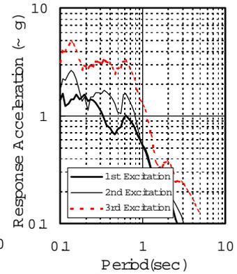
**Figure 5. Response Acceleration of Input Shaking Motion (5%)**
