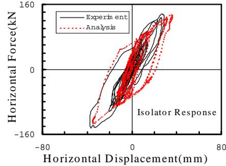
**(c) Seismic Isolator**
