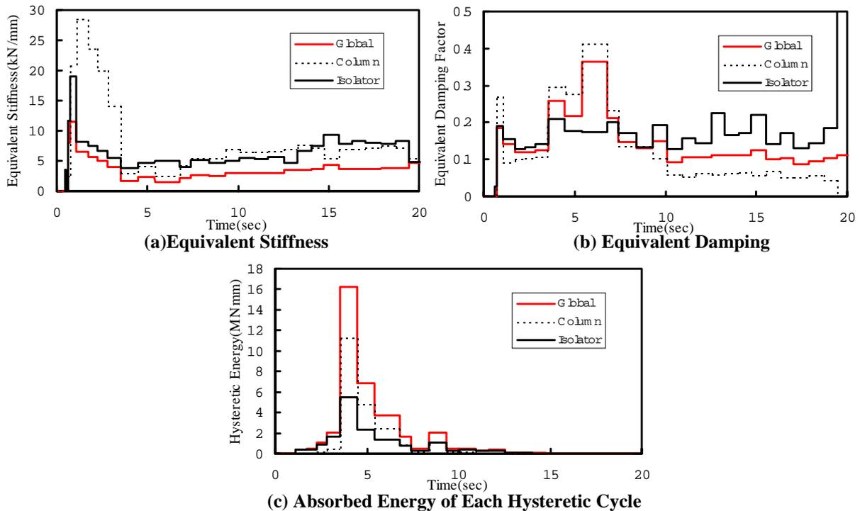
Figure 8. Time History of Equivalent Stiffness, Equivalent Damping, and Absorbed Energy of Each Cycle of the 1st Excitation
