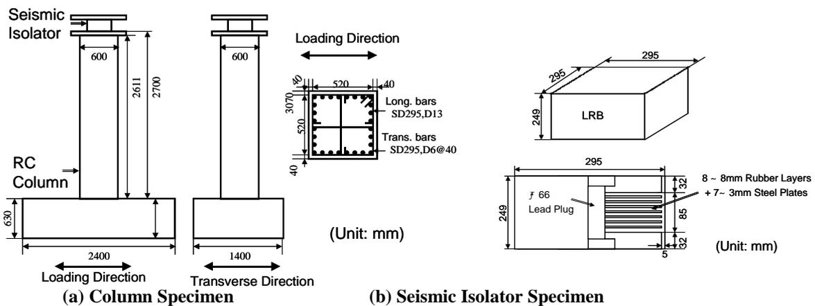
Figure 2: Column and Seismic Isolator Specimen
