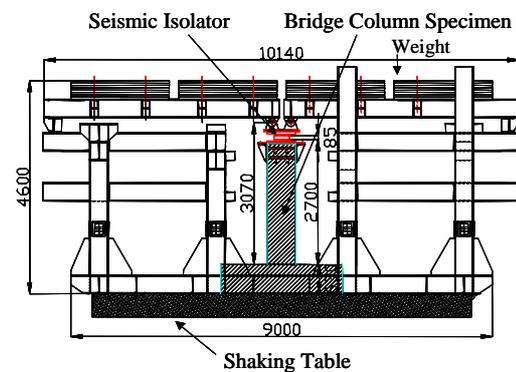
Figure 1: Shaking Table Set Up
