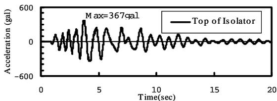
**(a) Top of Seismic Isolator**
