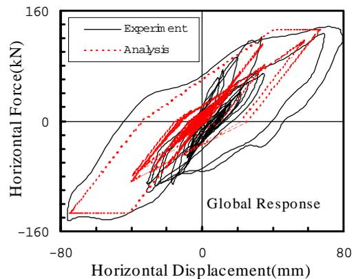
**Figure 13. Comparison between the Experimental and Analytical Results (Equivalent 1DOF Analysis: Equivalent damping was computed using equation (4))**
