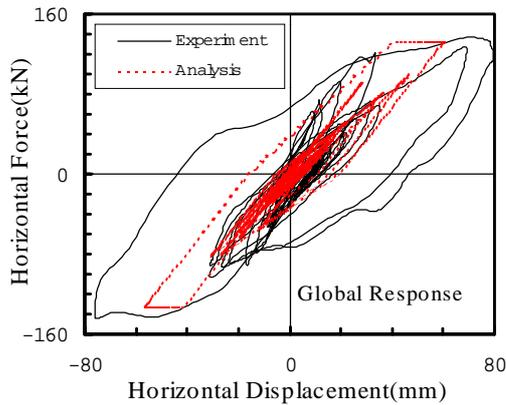
**Figure 12. Comparison between the Experimental and Analytical Results (Equivalent 1DOF Analysis: Equivalent damping was computed using equation (3))**
