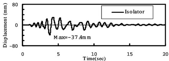
**(c) Relative Displacement of Seismic Isolator**
