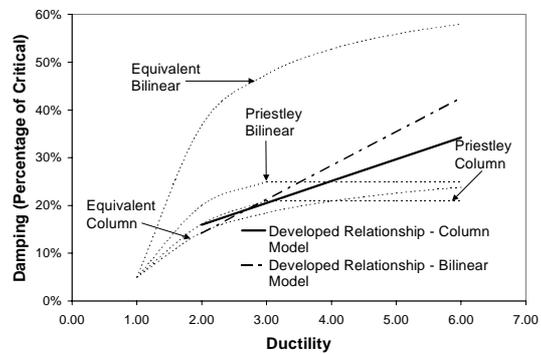
**Fig. (2) Damping vs. Ductility**
