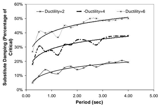
**Fig. (3) Substitute Damping Elastoplastic Model – Normalised El Centro**
