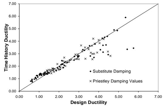
**Fig. (8) Comparison of Design Results (Stiffness Degrading Column Model)**
