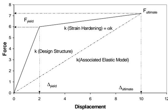
**Fig. (1) The Design Structure & The Associated Elastic Model in DDBD**
