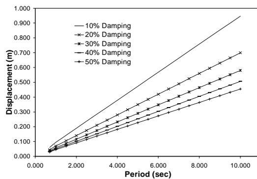
**Fig. (4) NZS4203: 1992 Elastic Design Displacement Spectra**
