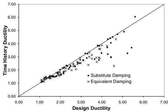
**Fig. (7) Comparison of Design Results (Stiffness Degrading Column Model)**
