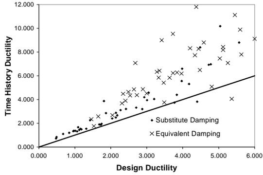
**Fig. (5) Comparison of Design Results (Elastoplastic Model)**
