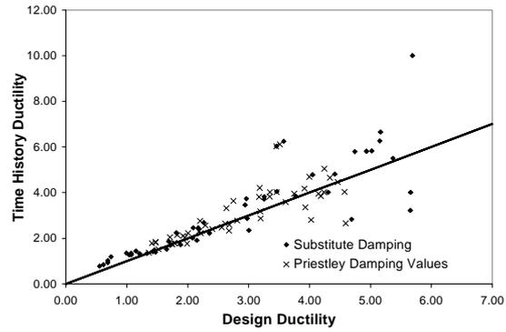
**Fig. (6) Comparison of Design Results (Elastoplastic Model)**
