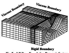
Fig.-7 3-D Dam-Foundation-Reservoir System Model with Non-reflective Boundary
