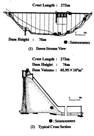
Fig.-2 Shape of Existing Concrete Gravity Dam and Arrangement of Seismometer
