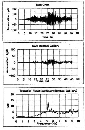
Fig.-3 Observed Earthquake Motions at the Kushiro-oki Earthquake and Transfer Function
