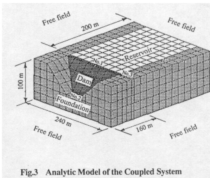
**Fig.3 Analytic Model of the Coupled System**
