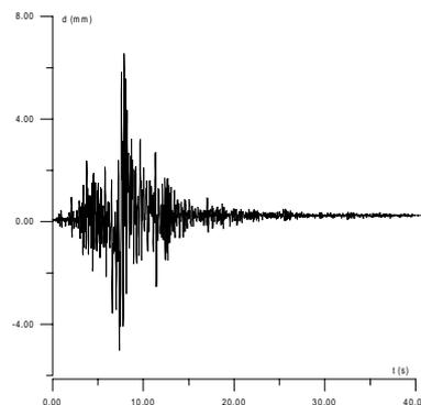
**Figure 9(a) SDOF model used for dynamic analysis (ISMES Laboratories, Italy). (b) Top frame displacement under 1.8 scaled Loma Prieta Earthquake**
