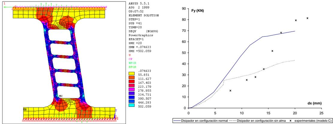
**Figure 7(a) Finite element model SLD without web, at 20 mm displacement, with von Mises stress distribution. (b) Numerical - experimental comparison for  $F_y - d_x$  for C device**
