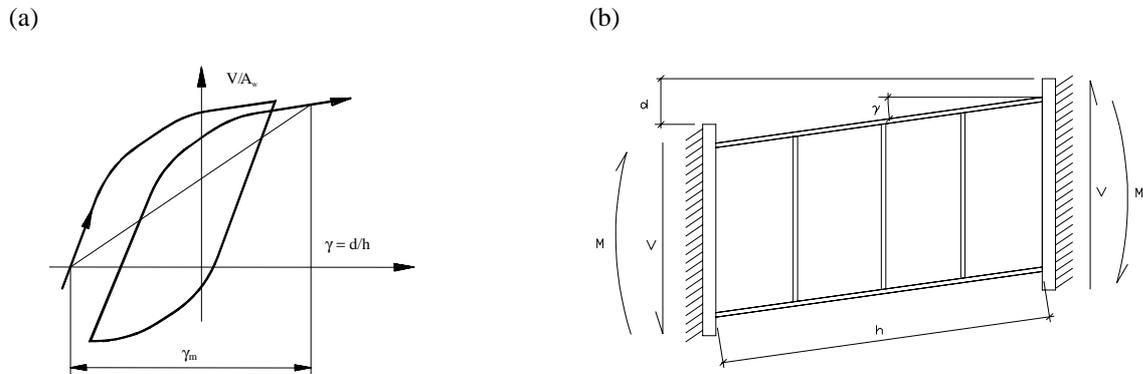
**Figure 5 (a) Average shear strain - link deformation angle relationship. (b) Deformed shear link element.**
