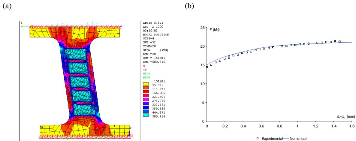
**Figure 6(a) Finite element model for thick SLD with von Mises stress distribution at  $d_x=20$ mm. (b) Numerical - experimental comparison for  $F_x - d_{x,plastic}$  for C device**
