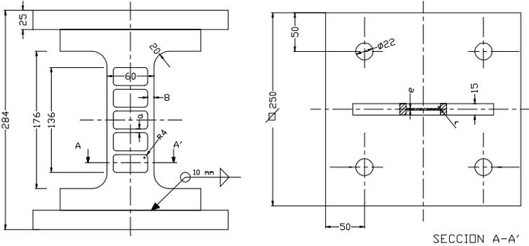
Figure 1. Shear link dissipator manufacturing drawings used for the tests specimens
