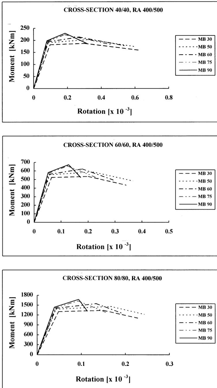
Figure 3. Moment-rotation relationship for different cross-section
