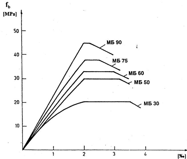
Figure 1.  $\sigma$ - $\epsilon$  diagram for different class of concrete
