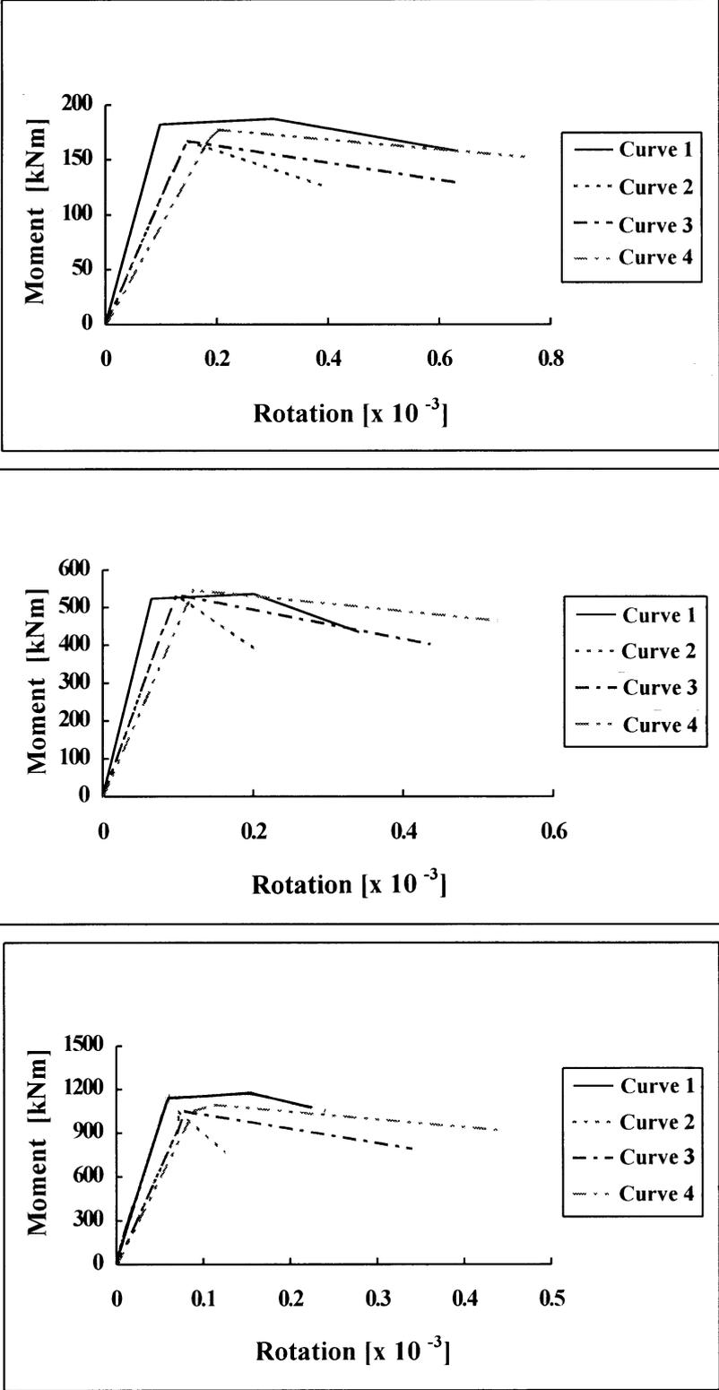
Figure 4. Moment -rotation relationship for comparative analysis of cross-sections
