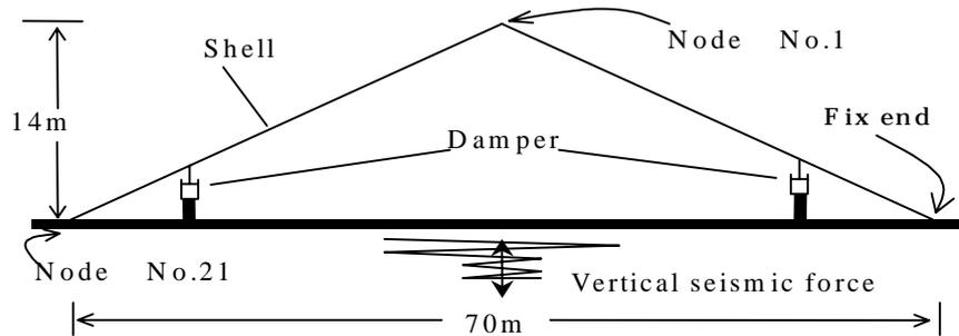
**Fig. 2 Conical shell with dampers**
