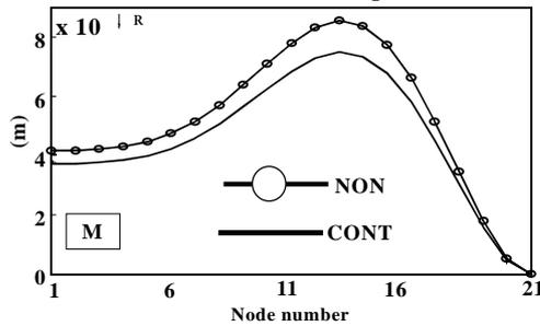
Fig. 6 Vertical displacements  $u^*$
