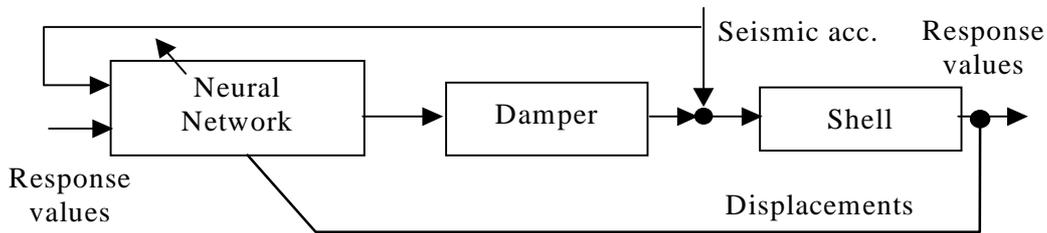
**Fig.1 Flow of vibration control**
