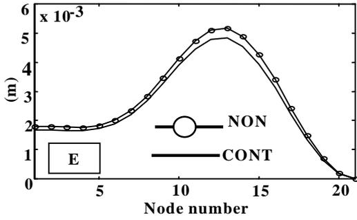
Fig. 8 Vertical displacements  $u^*$
