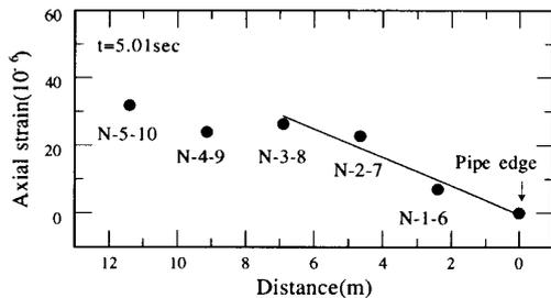
**Fig. 17: Axial strain distribution in experiment A4**
