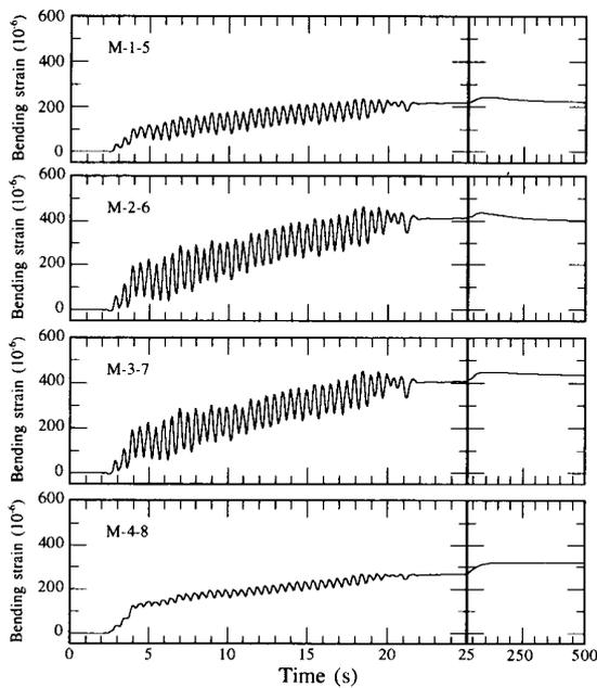
**Fig. 12: Time histories of bending strain on the pipe in experiment T1**
