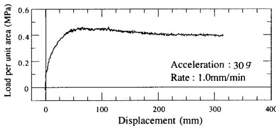
**Fig. 4: Load-displacement relationship in the transverse horizontal load experiment**
