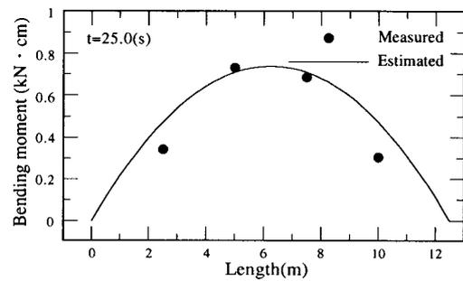
**Fig. 13: Measured and estimated bending moment along pipe axis in experiment T1**
