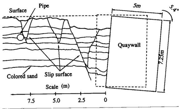
**Fig. 10: Sketch at the cross section after experiment T1**
