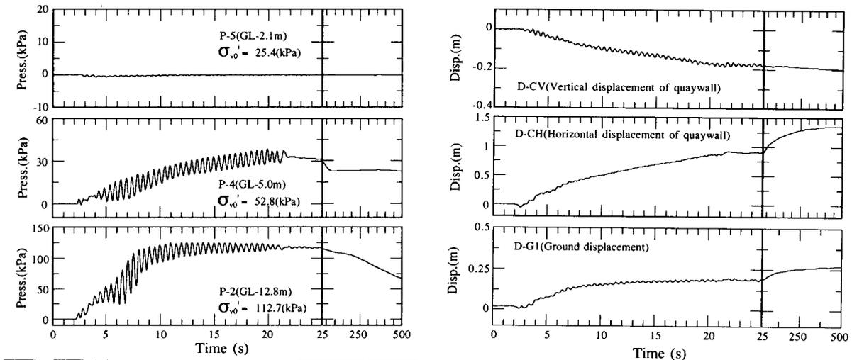
**Fig. 8: Time histories of pore water pressure in experiment T1**      **Fig. 9: Time histories of quaywall and ground surface displacement in experiment T1**
