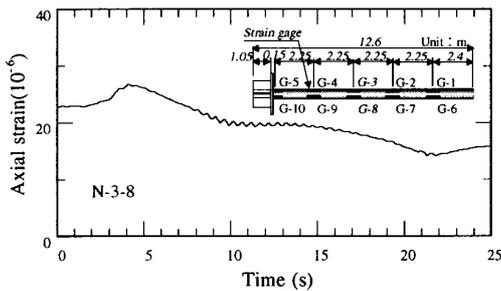
**Fig.16: Time history of axial strain in experiment A4**
