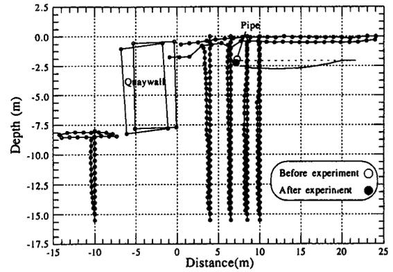
**Fig. 11: Ground displacement at the cross section after experiment T1**
