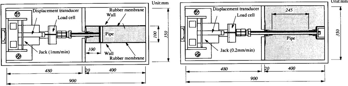
**Fig. 1: Plan view of the forced pipe displacement model for the transverse horizontal load**
