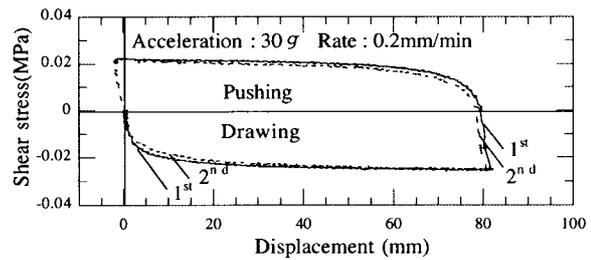
**Fig. 5: Load-displacement relationship in the axial load experiment**
