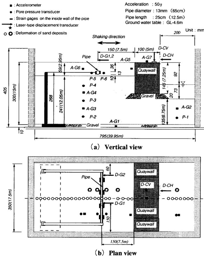
**Fig. 6: Liquefaction-induced ground displacement model for the transverse horizontal load**
