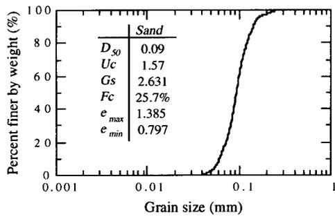
**Fig. 3: Grading curve and physical properties**
