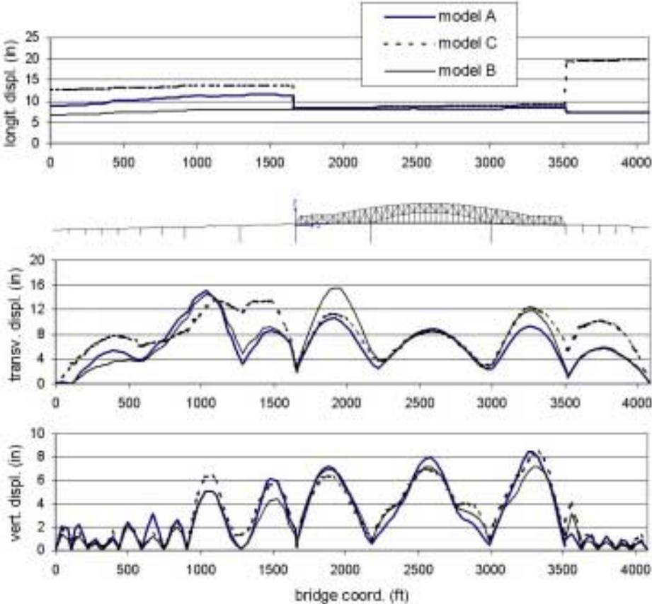
Figure 4. Max. displacements along the deck
