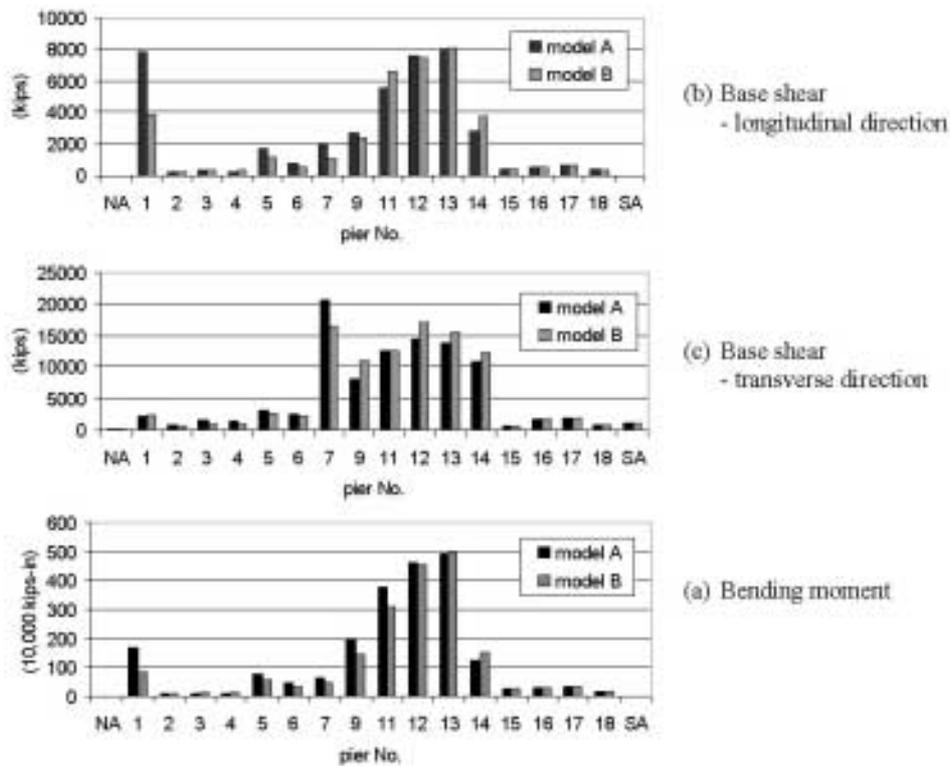
Figure 4. Reaction Forces at the base of each pier
