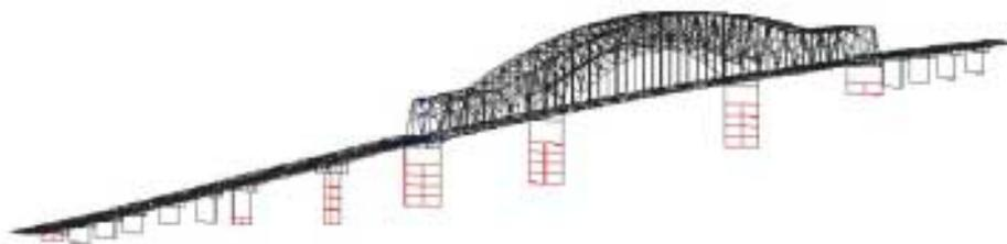
Figure 2. FE model of the bridge.
