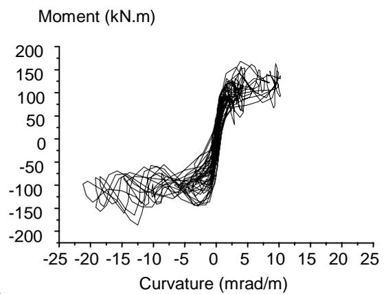
**Figure 8-Moment-curvature relationship (Last test of CAMUS II)**
