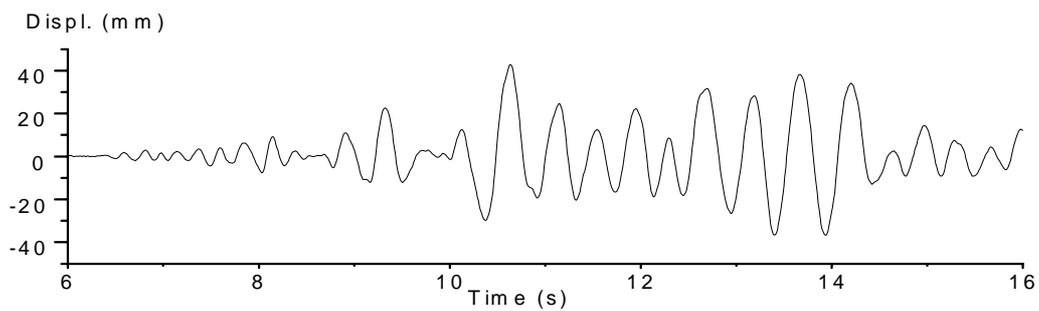
**Figure 6- Evolution of top displacement (last test of CAMUS II)**
