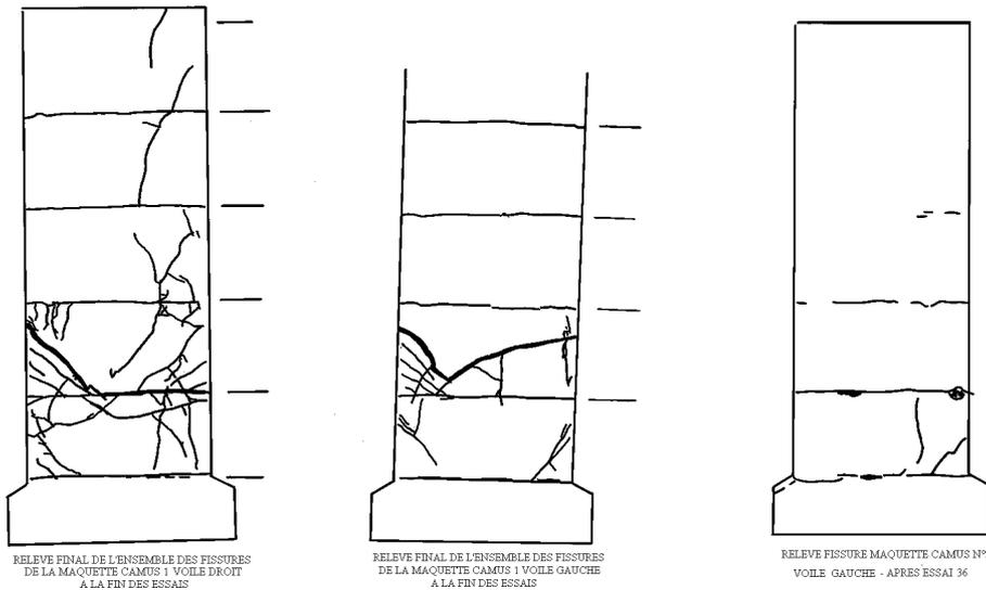
**Figure 4- Cracking at the end of CAMUS I tests**      **Figure 5- Cracking at the end of CAMUS II tests**
