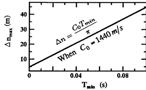
**Fig.3 Relationship of the Maximum Mesh Size With the Minimum Period and Wave Velocity**
