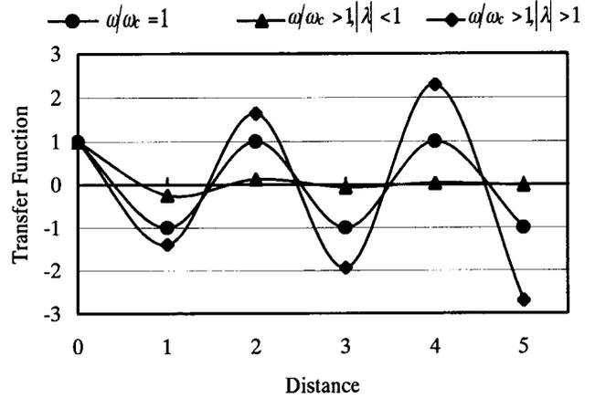
**Fig.2 Relationship of Distance from Dam and Transfer Function**
