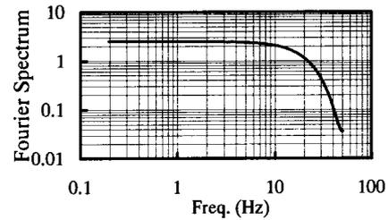
**Fig. 5 Input Wave (Gauss Pulse)**
