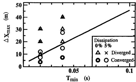
**Fig. 7 The Stability of the Dam Response Effected by the Maximum Mesh Size and Minimum Period**
