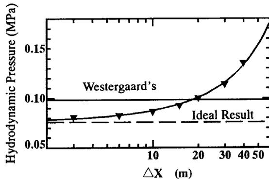
**Fig. 6 Variation of Hydrodynamic Pressure Result from the Modification of Mesh Sizes**
