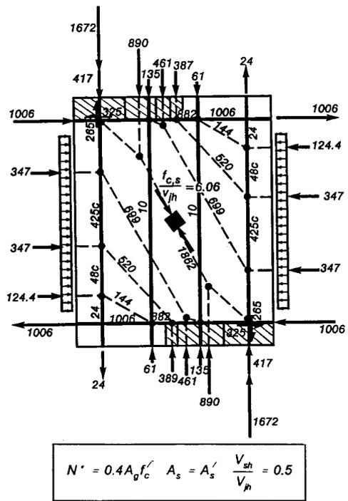
Figure 3: Effect of column axial load on the stress ratio  $f_{c,s} / v_{jh}$
