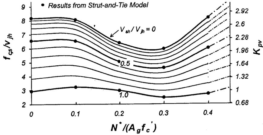
Figure 4: Combined effect of ratios  $N^*/(A_g f_c')$  and  $V_{sh}/V_{jh}$  on the stress ratio  $f_{cs}/v_{jh}$
