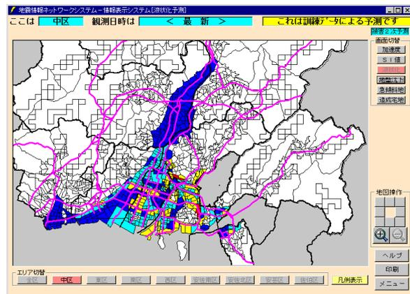
Fig.11: Liquefaction potential distribution
