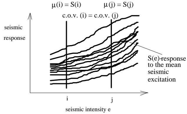
**Figure 4: Concept of 'mean seismic excitation'**
