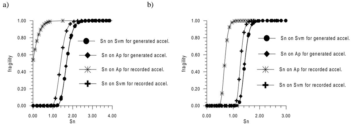
**Figure 5: Fragilities of FRSR and FRS on different seismic intensity parameters:**
