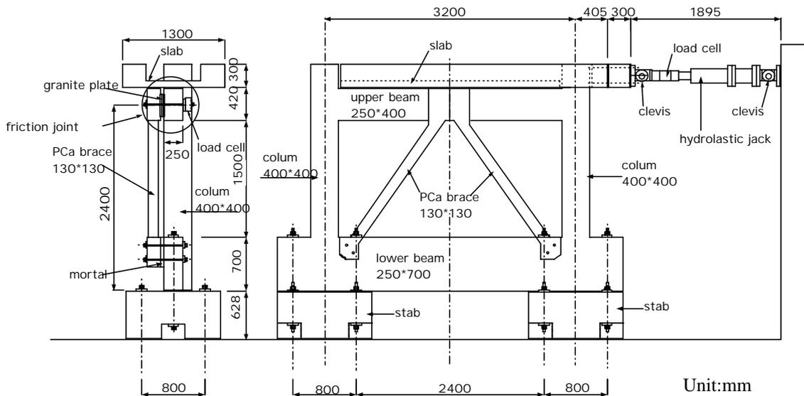
**Fig.6 lateral seismic loading test**
