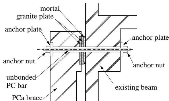
**Fig.2 friction joint connected to upper beam**
