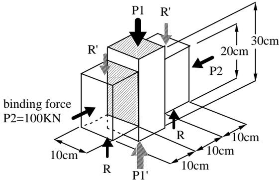
**Fig.4 Friction tests of granite columns**
