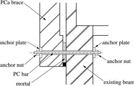
**Fig.3 fixed joint connected to lower beam**
