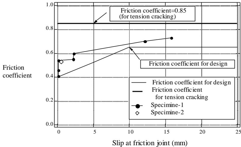
**Fig.9 comparison of design friction coefficient and observed friction coefficients**
