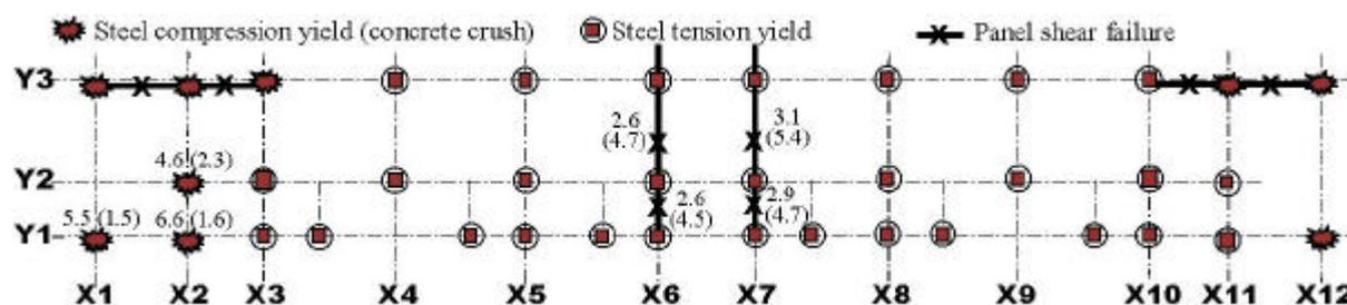
Figure 9: Predicted damage distributions in structural model with multi-rigid diaphragms
