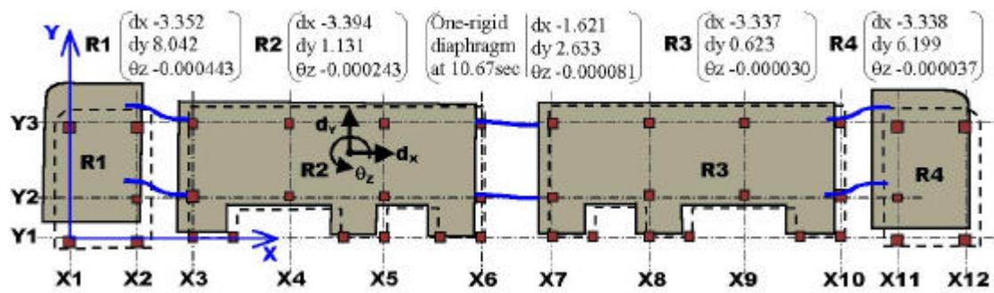
Figure 7: Top floor displacement at peak responses (at 10.25 sec)
