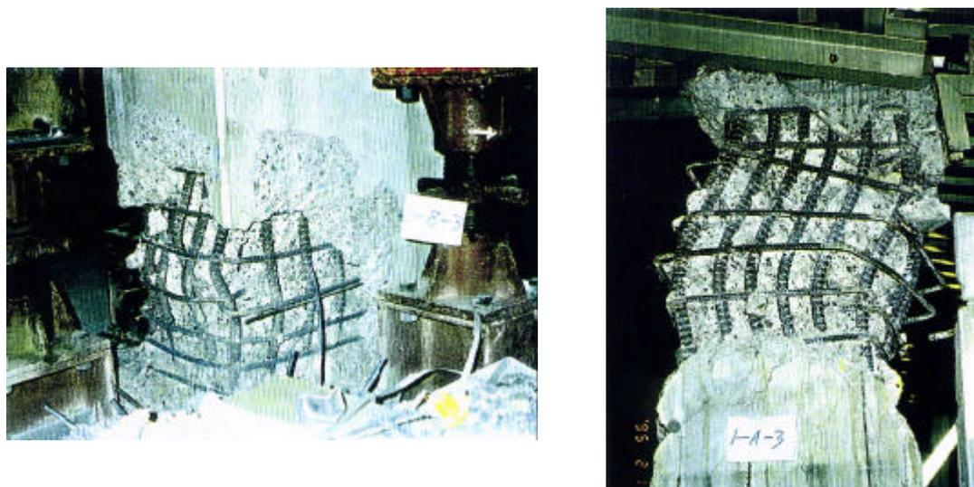
**Figure 3: Sample of the damage of 1st-story columns (left: column base, right: column top)**
