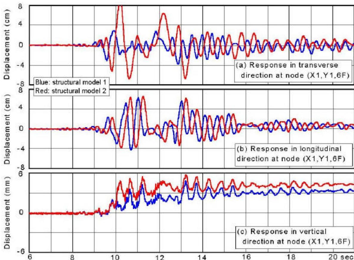
Figure 8: Comparing the responses at structural node predicted by the two structural models
