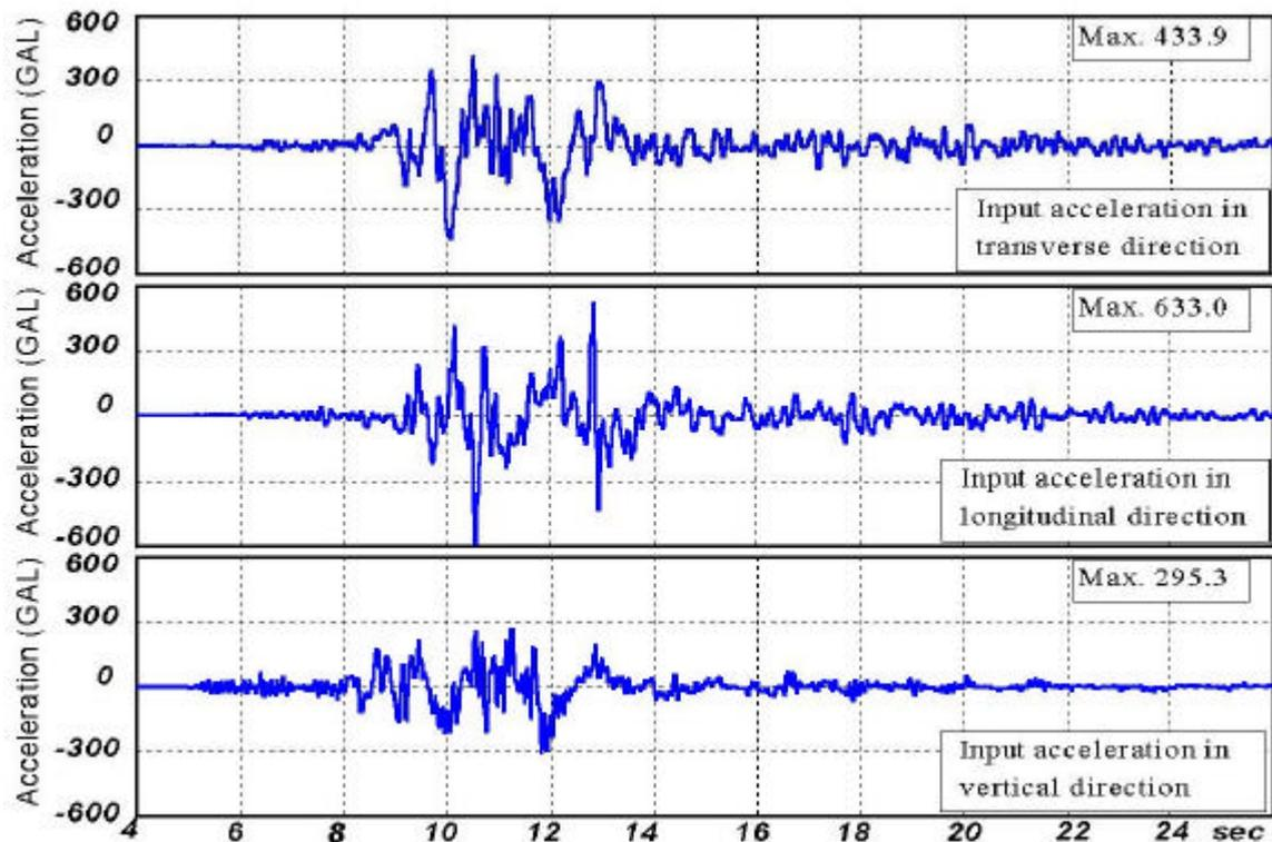
**Figure 5: Input accelerations evaluated from nearby records during the earthquake**
