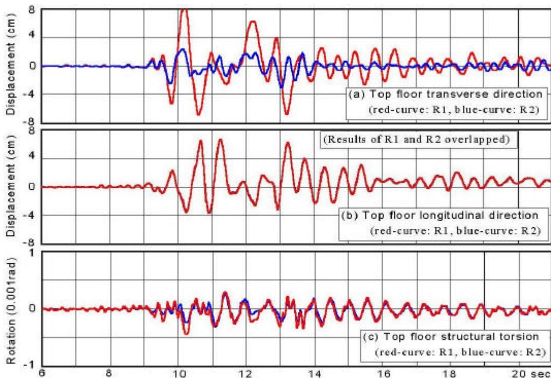
Figure 6: Displacement responses at top floor level of the multi-rigid diaphragm structural model
