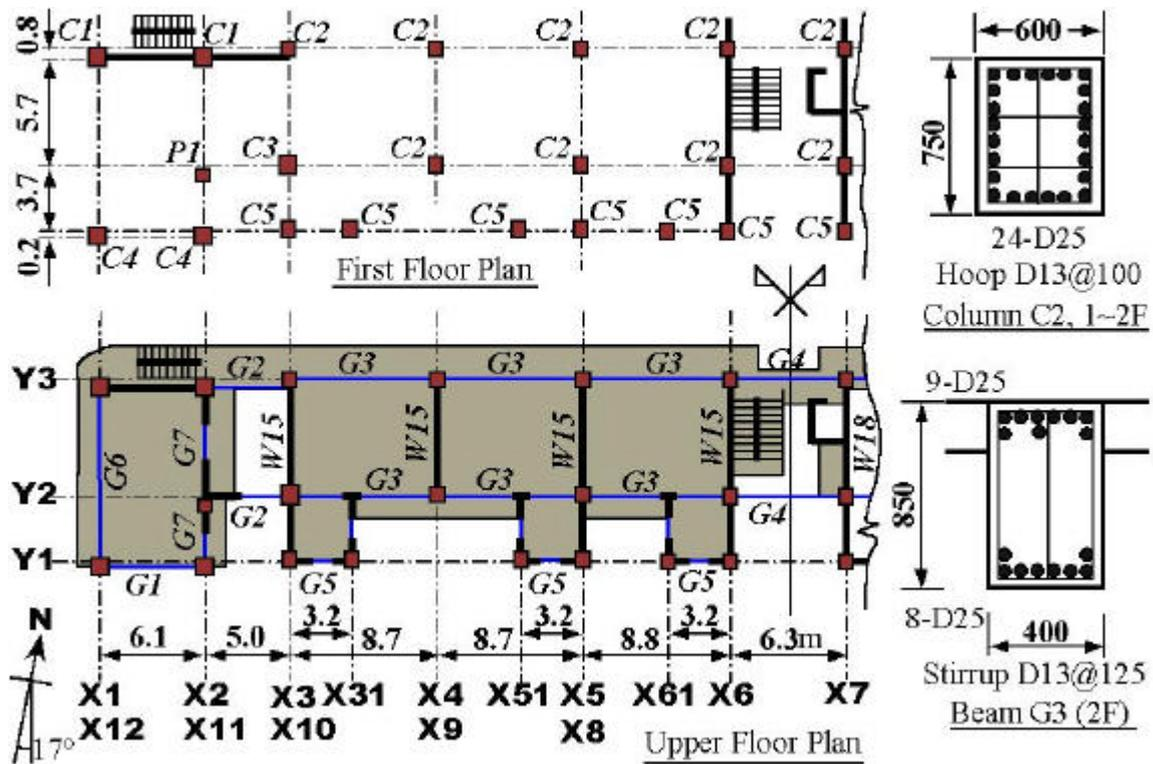
Figure 1: Typical floor plan and member sections of the analyzed building structure
