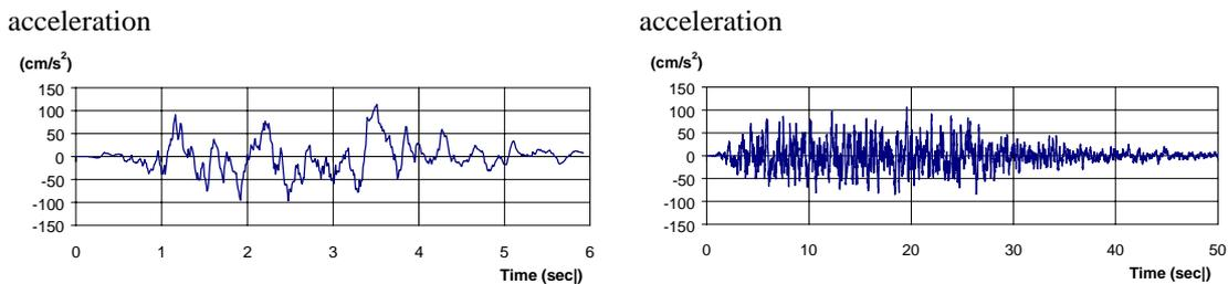
**Figure 5: Sample of generated short duration (left) and long duration (right) acceleration records for Tokyo**
