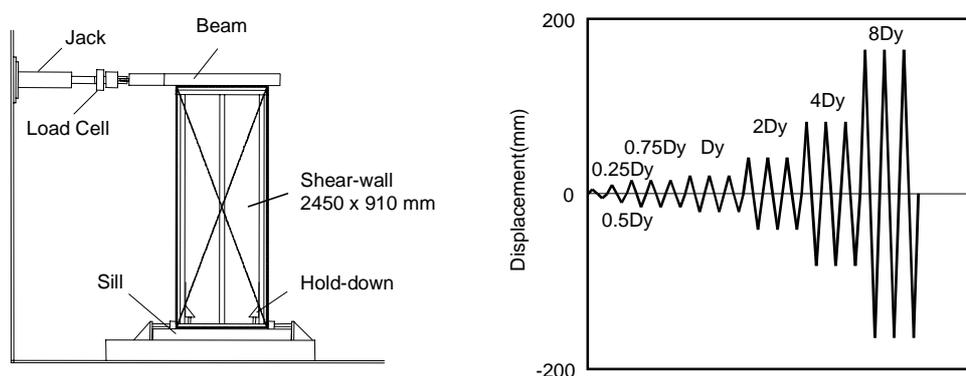
**Figure 1: Static-cyclic test setup and loading sequence of BRI shear wall (from Kawai [1998])**
