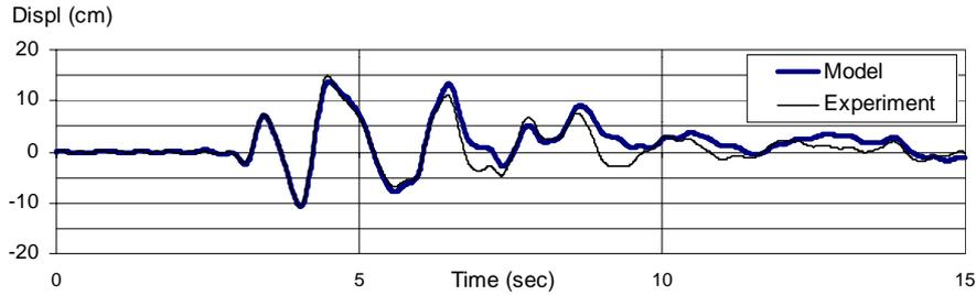
**Figure 3: Experimental (from PSD test) and fitted displacement response of timber shear wall under a 0.6g Kobe earthquake record**
