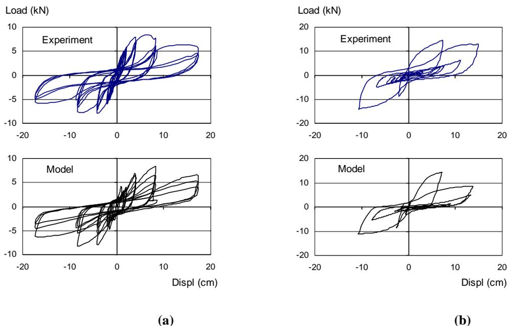
**Figure 2: Experimental and fitted hysteresis loops for (a) static-cyclic test and (b) pseudo-dynamic test**
