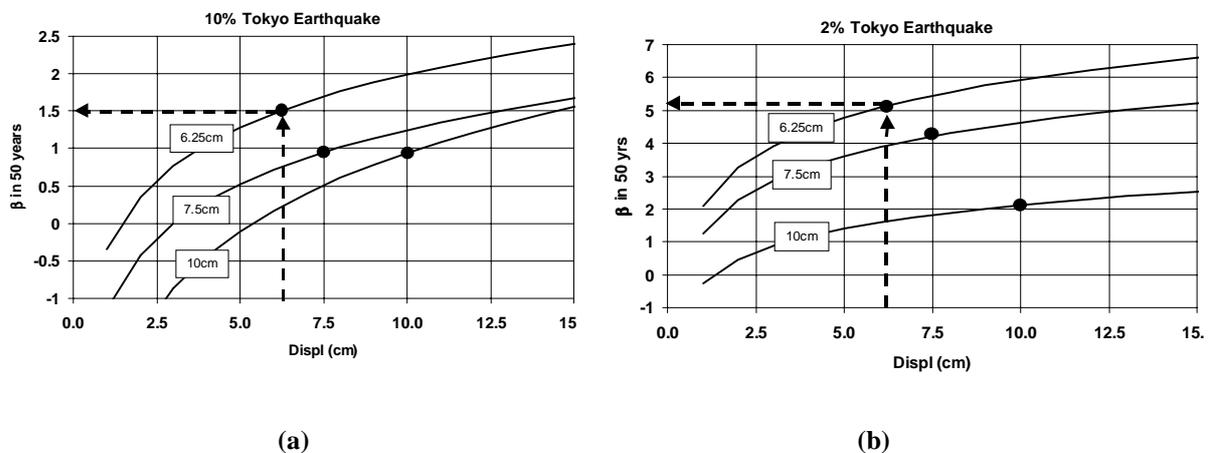
**Figure 7: Reliability curves for the shear wall with sustainable mass obtained from Tokyo earthquake records with: (a) 10% probability of exceedance, and (b) 2% probability of exceedance in 50 years**
