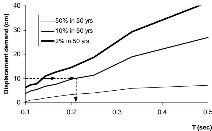
**Figure 6: Displacement spectra for shear wall under three levels of excitation**
