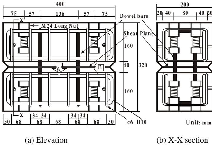
Figure 1: Specimen dimensions and reinforcement arrangement
