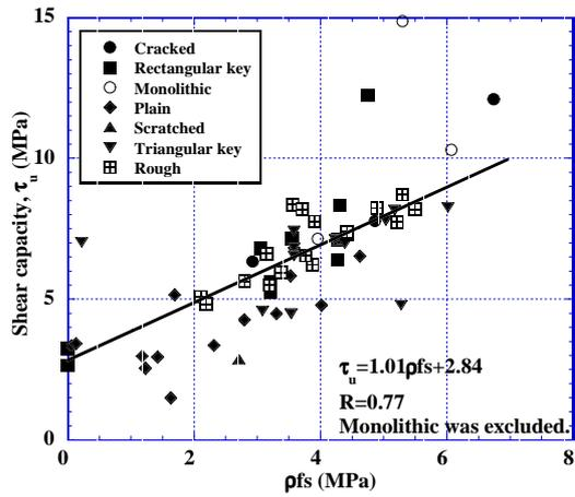
Figure 8: Shear capacity - $\rho f_s$  relations
