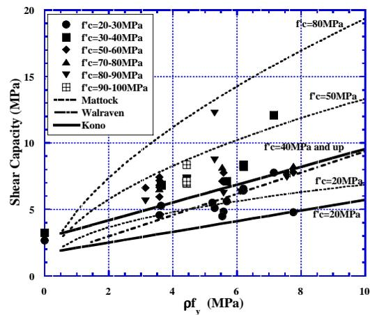
Figure 11: Shear capacity -  $\rho f_y$  relations
