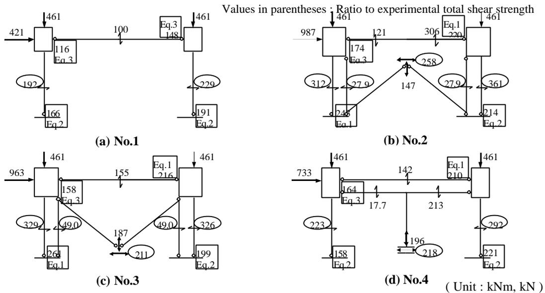
**Fig.9: Stress Diagram (Calculated using simplified formulas)**
