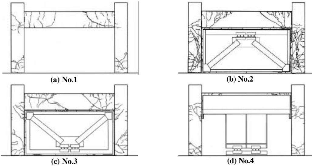
Fig.6: Crack distributions (Story drift angle: 1/100 rad)
