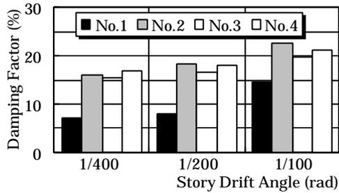
Fig.7: Equivalent viscous damping factors
