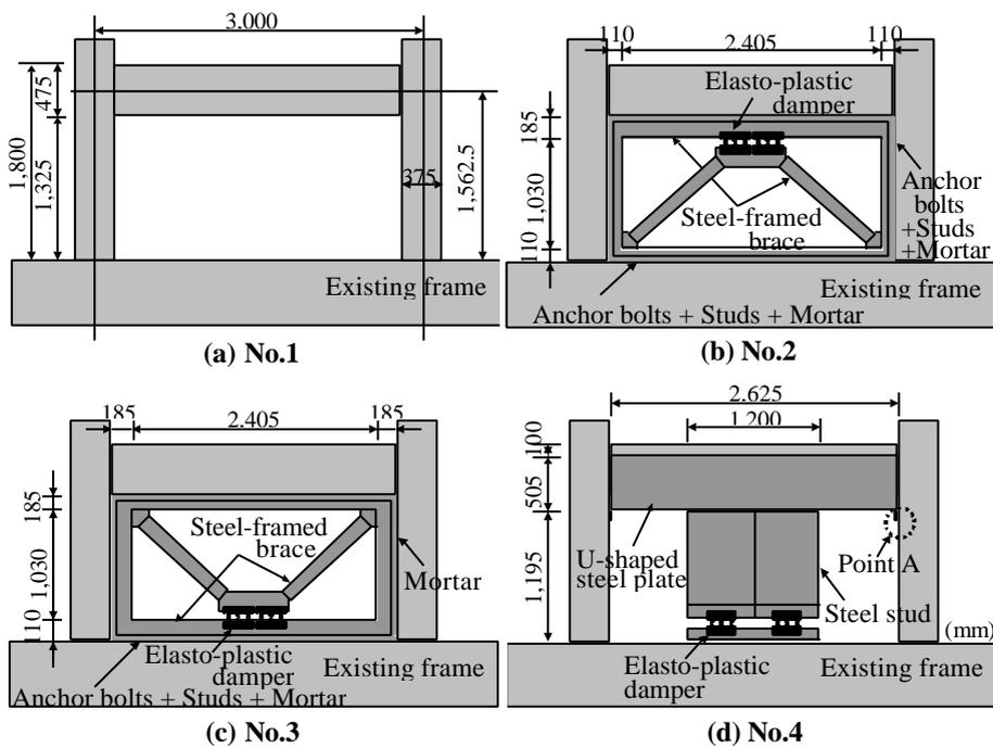
Fig.2: Test specimens
