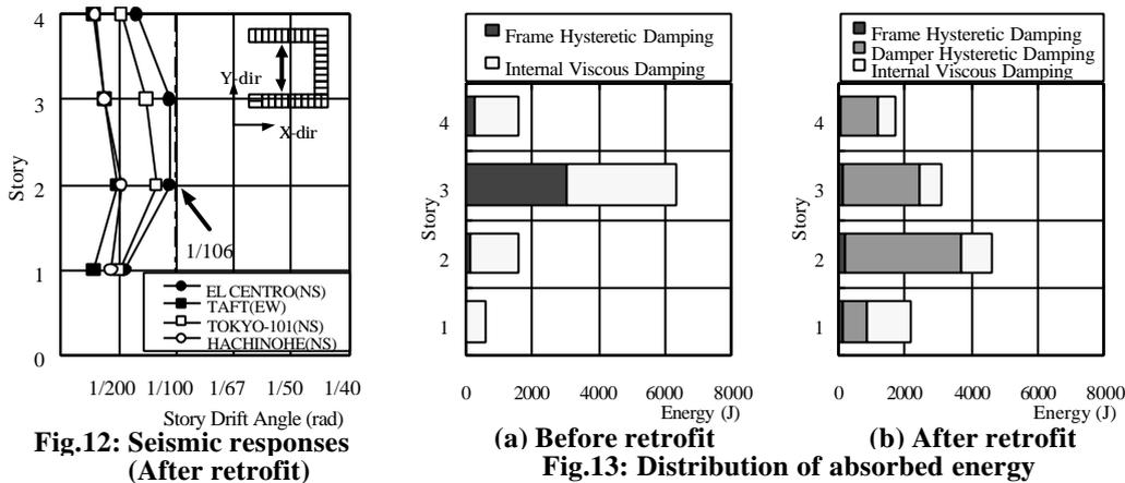
Fig.12: Seismic responses (After retrofit)
