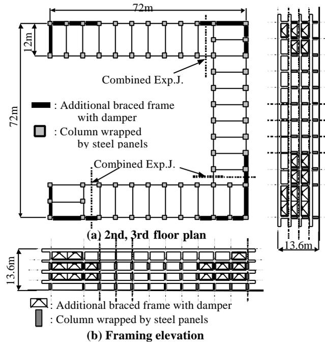
**Fig.11: Locations of reinforcing frame**
