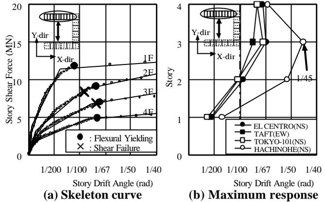
**Fig.10: Seismic responses (Existing building)**
