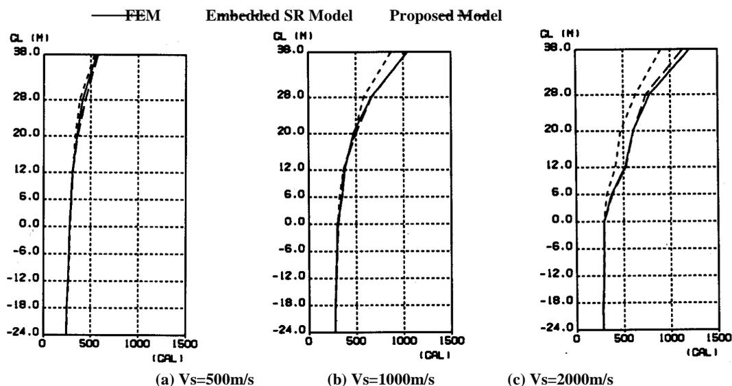
Fig.-10 Maximum Acceleration of Structure
