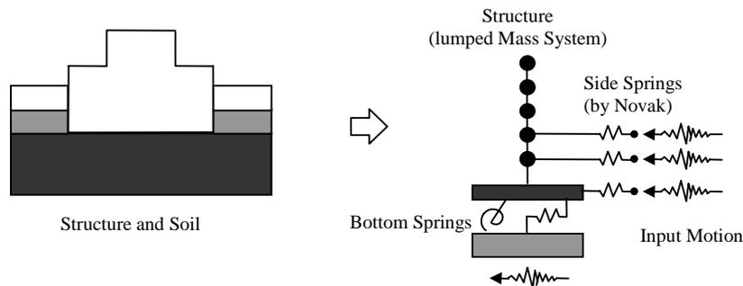
**Fig.-1 Concept of Embedded SR Model**
