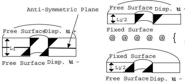
Shear Spring for Layer(  $L_i$  ) Springs Shown by Harada
