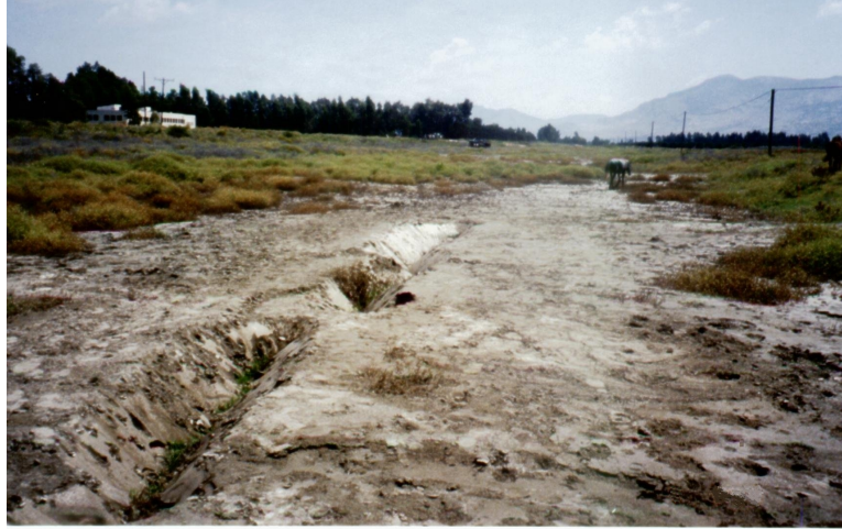
Figure 5: A major sand boil formation in the epicentral area.
