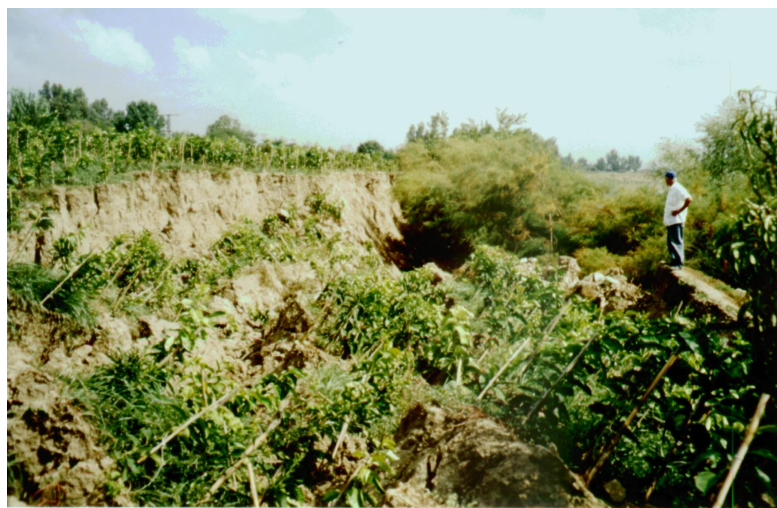
Figure 6: Lateral spreads in an orchard along Ceyhan River near Abdioglu.
