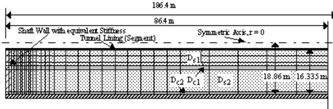
Figure 10: Discretization of axisymmetric finite element mesh
