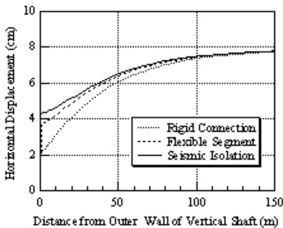
Figure 11: Horizontal Displacement of tunnel lining during compressive deformation
