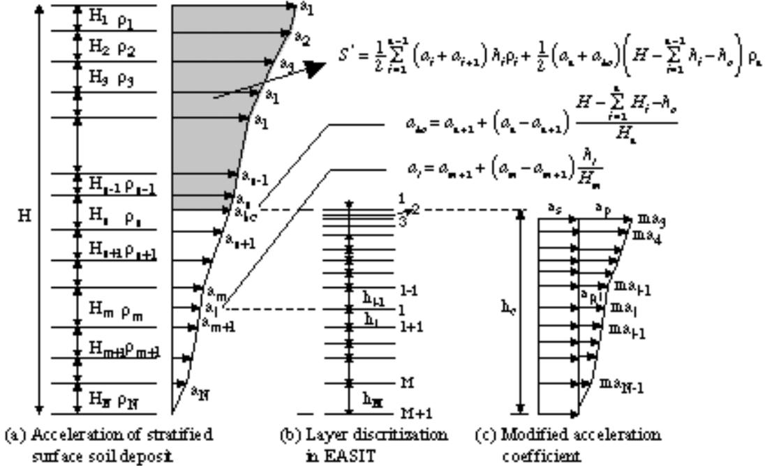
Figure 5: Process of acceleration conversion from stratified surface soil deposit to the axisymmetric model
