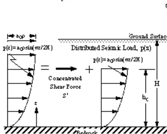
Figure 3: Method to apply seismic load
