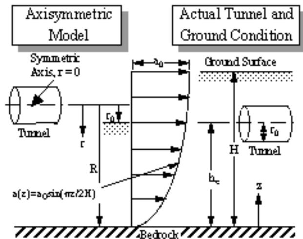
Figure 2: Coordinate of the axisymmetric model in comparison with actual condition
