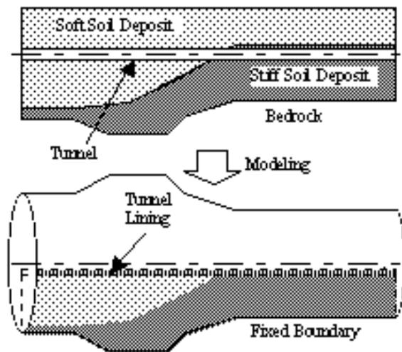
Figure 1: Schematic representation of the axisymmetric model
