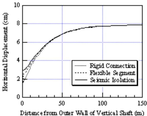
Figure 13: Horizontal Displacement of tunnel lining during tensile deformation
