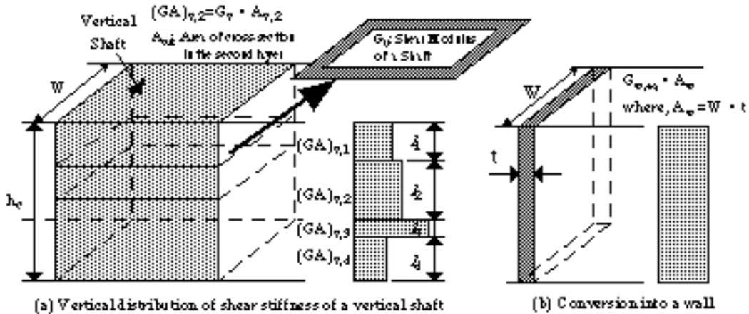
Figure 6: A schematic diagram to illustrate the conversion of a vertical shaft into a wall consisting of equivalent shear stiffness
