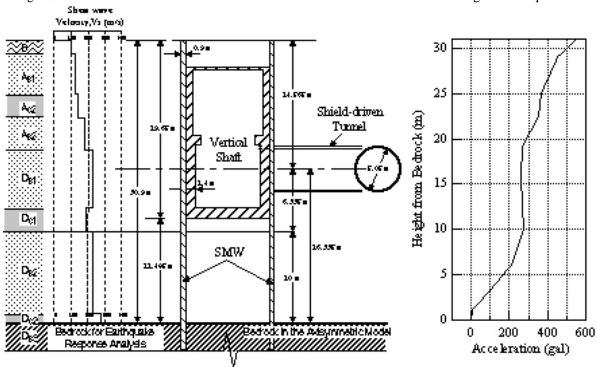
Figure 7: Ground and structure condition and loaded ground acceleration in numerical simulations
