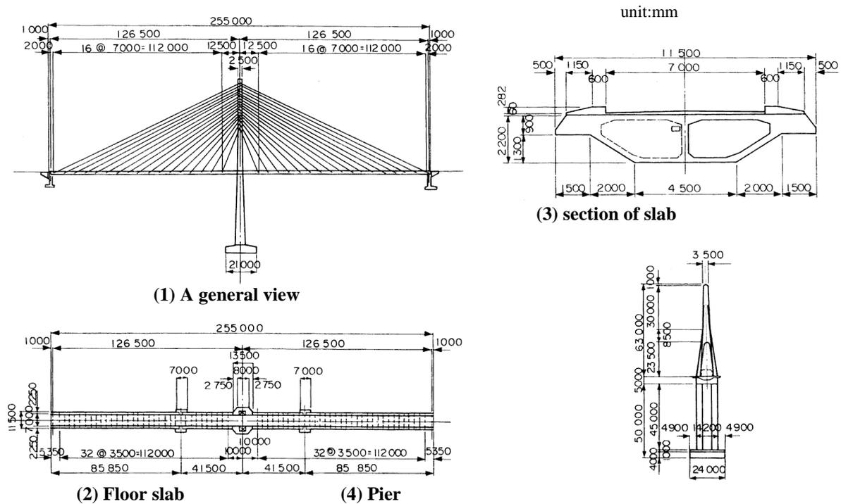
Figure 1: Parameter of the object CSB
