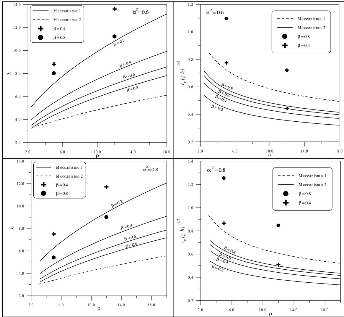
**Figure 2: Slenderness and normalised collapse acceleration of the façade subject to an impulsive out of plane force: comparison between the analytical expressions corresponding to the two failure mechanisms proposed and the values of the numerical analysis performed using a discrete element method.**
