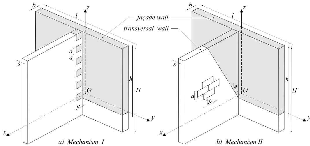
**Figure 1: Failure mechanisms: a) detachment of the façade from the lateral wall with a vertical crack at the abutment; b) overturning of the façade and part of the transversal wall with the formation of a diagonal crack.**
