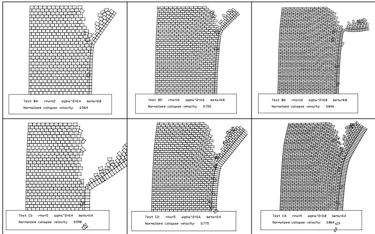
**Figure 3. Failure mechanisms and corresponding normalised collapse velocity of six identically-shaped transversal walls ( $H=9$  m,  $l=6$  m,  $s=50$ ), built of variously sized blocks, when varying the thickness ( $b = 25 : 50$  cm) and le length ( $l = 2.5 : 6$  m) of the façade.**
