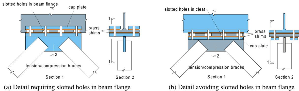
**Figure 3 Sliding connection configurations at junction of a brace and beam**
