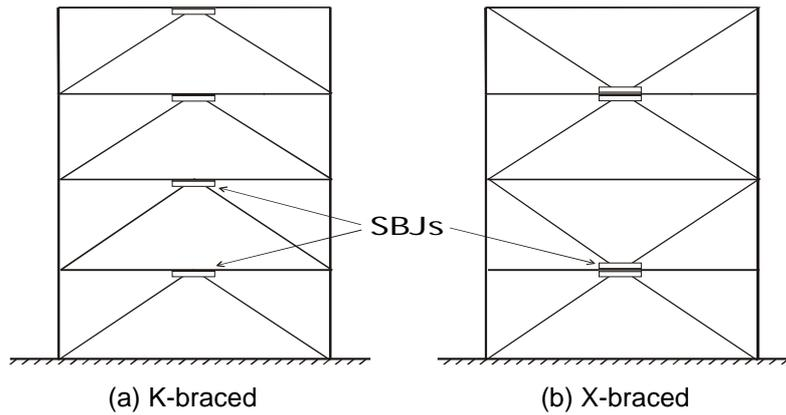
**Fig.5 K and X-braced configurations**
