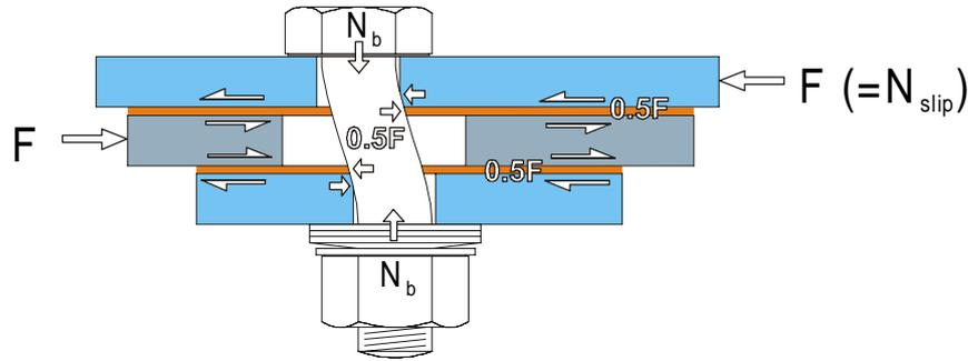
**Fig. 2 Asymmetric sliding joint**
