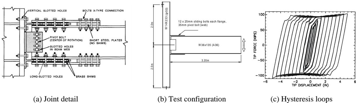
**Fig. 6 Rotational slotted bolted connection (RSBC) [Yang & Popov, 1995]**
