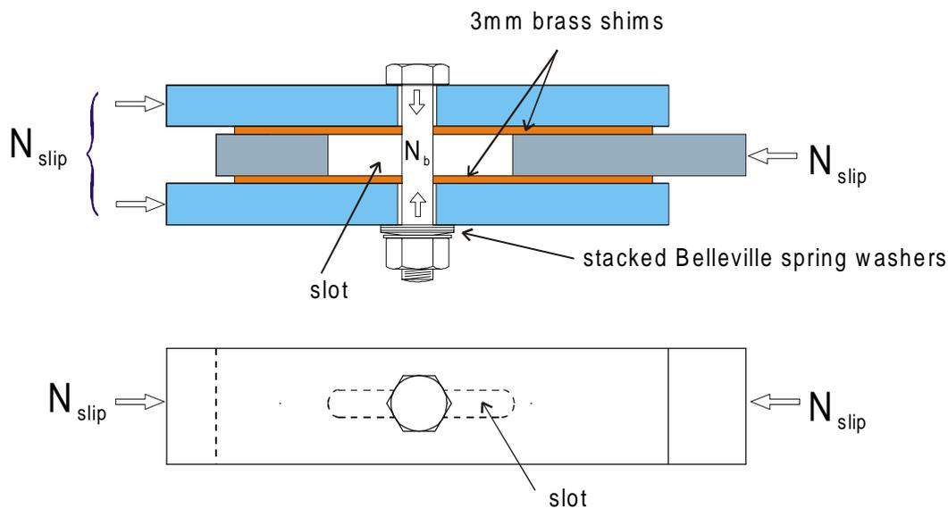
**Fig. 1 Basic sliding joint details**
