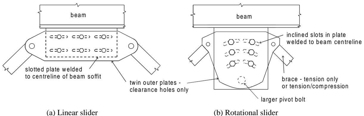
**Figure 4 Vertically oriented sliding interfaces for braced frame dissipators**
