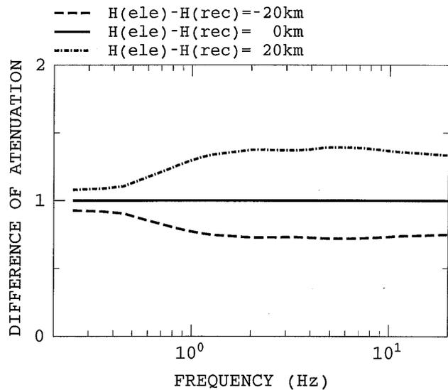
Figure 3: Difference of the attenuation of Fourier amplitude for different focal depth based on
