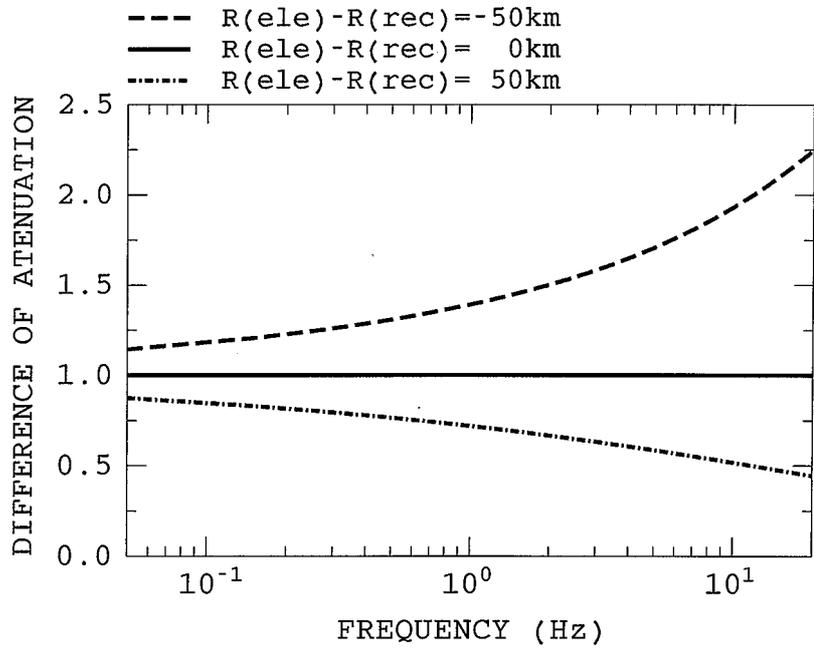
**Figure 1: Difference of the attenuation of Fourier amplitude for different focal distance based on the  $Q$  factor**
