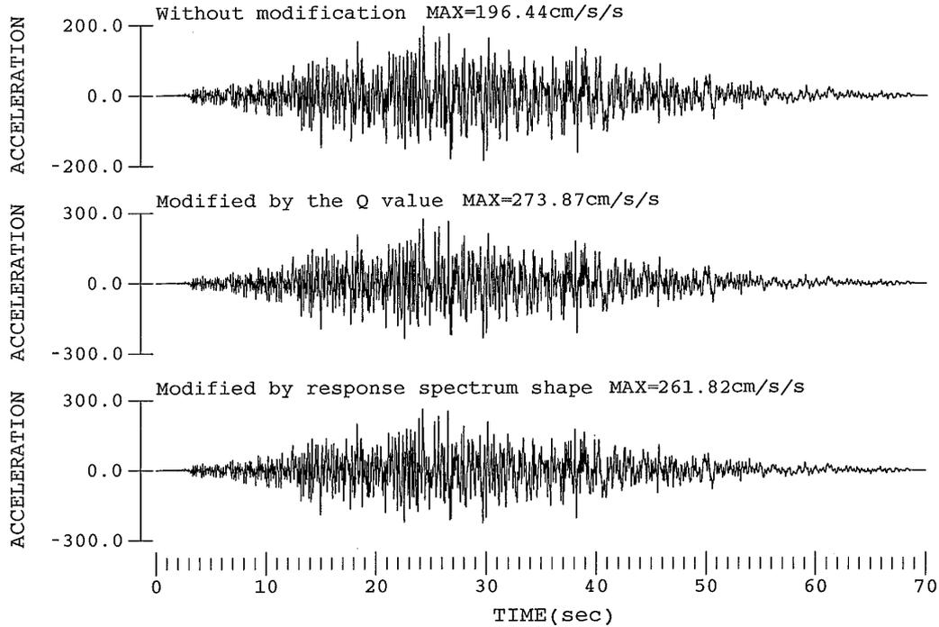
**Figure 6: Synthesized ground motions with and without frequency contents modification**
