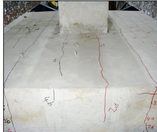
Figure 7: 2nd interior specimen. Photo shows the absence of torsional cracking
