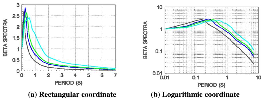
**Figure 1 Average  $\beta$  Spectrum of Each Group with 5% Damping Ratio**
