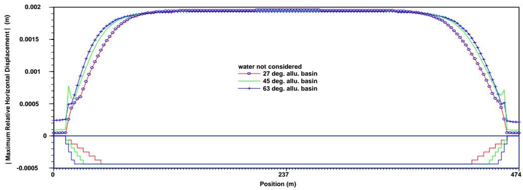
**Figure 6: Peak horizontal displacement for basin with different slopes (PGA=0.05g)**
