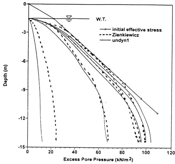
Figure 2: Comparison for distribution of excessive pore water pressure
