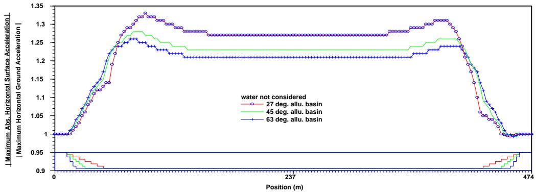
Figure 5: Peak horizontal acceleration ratio for basin with different slopes (PGA=0.2g)
