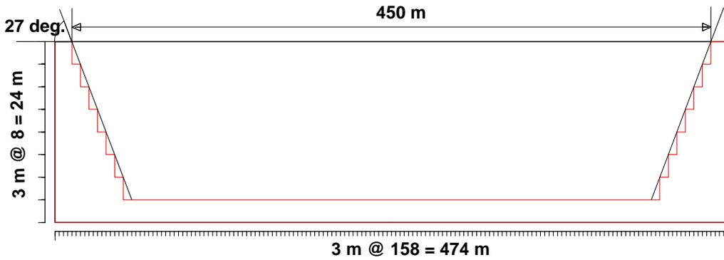
Figure 3: Basin model used for analysis
