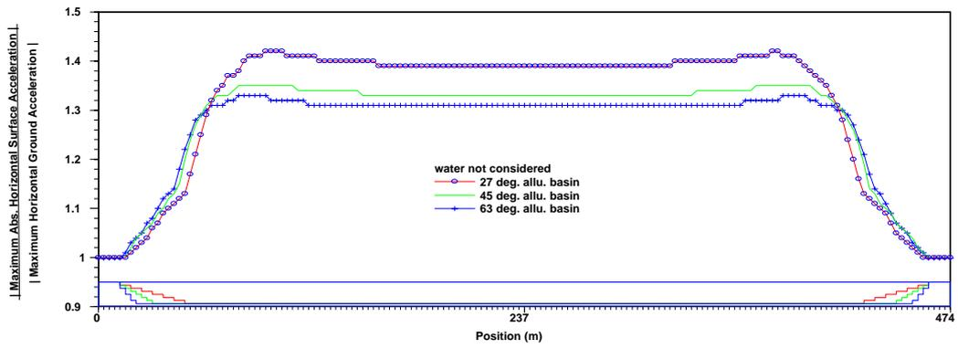
Figure 4: Peak horizontal acceleration ratio for basin with different slopes (PGA=0.05g)
