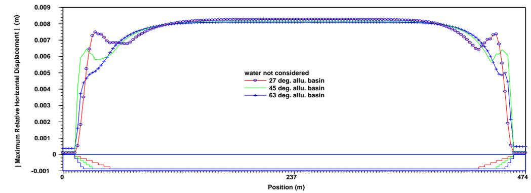
**Figure 7: Peak horizontal displacement for basin with different slopes (PGA=0.2g)**
