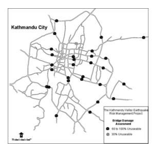
Figure 2. Estimated potential damage to bridges in Kathmandu City.
