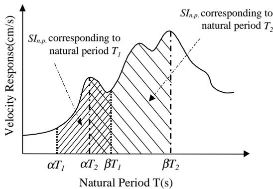
**Figure 1: Conceptual Diagram of Proposed  $SI_{n,p}$ .**
