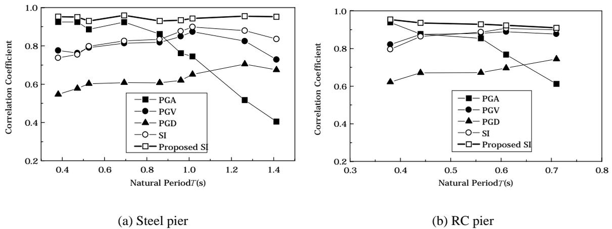
**Figure 5: Correlation coefficient against maximum response displacement**
