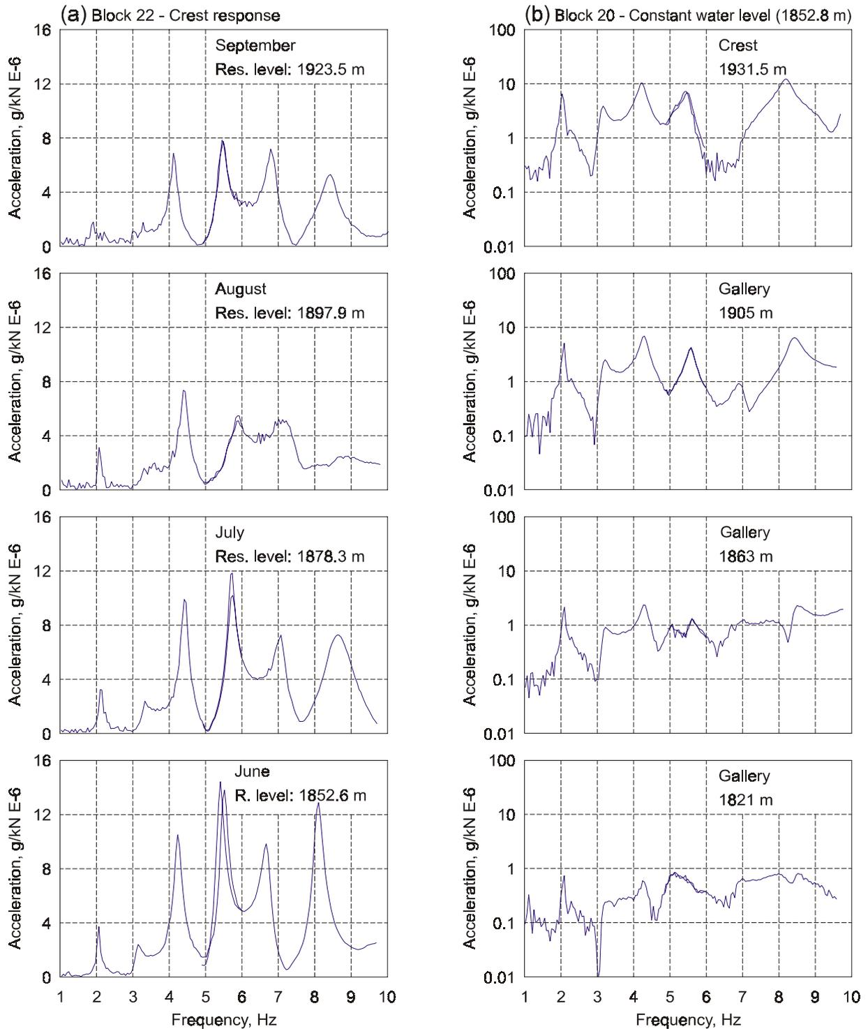
Figure 4: Frequency responses for blocks (a) 22 and (b) 20
