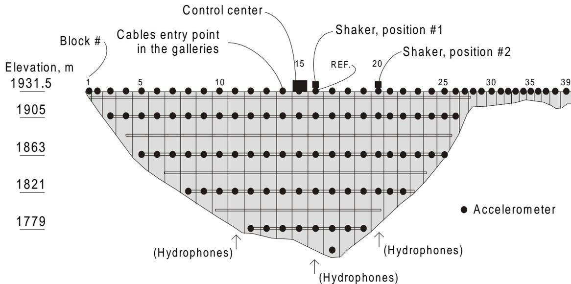
**Figure 3: Experimental setup**
