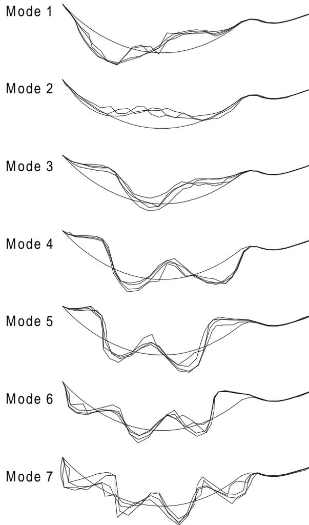
**Figure 5: Experimental resonance shapes**
