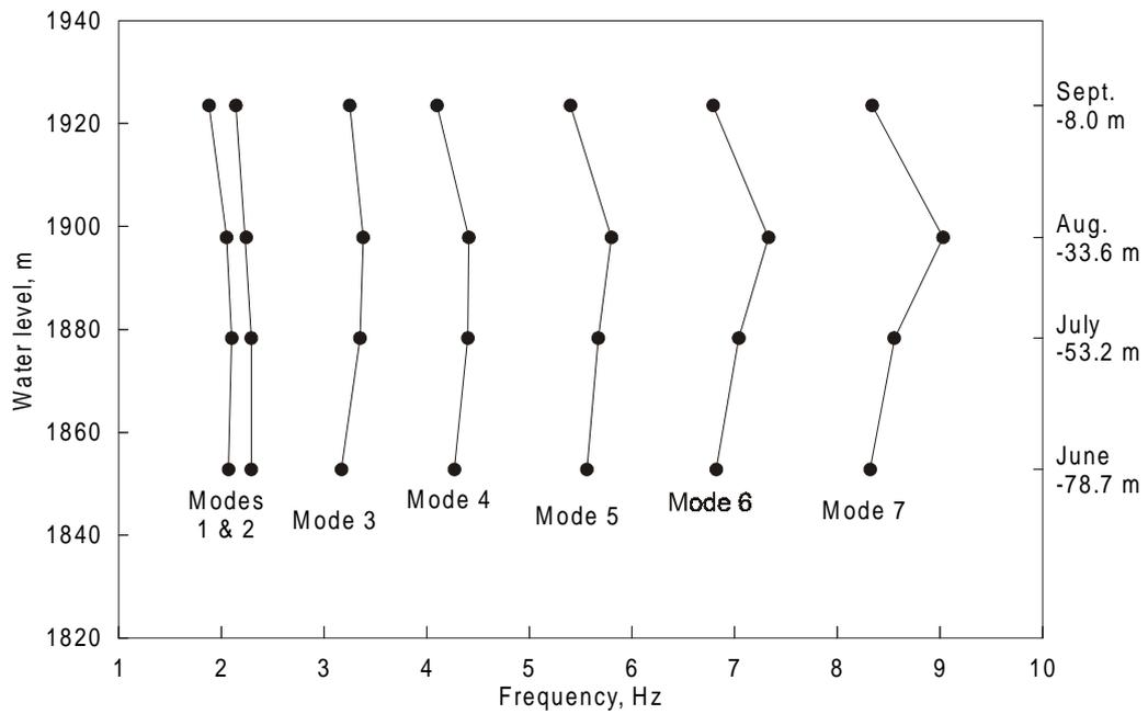
**Figure 6: Effect of water level on resonant frequencies**
