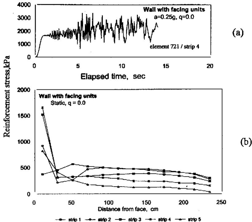
Figure 5. (a) Tensile stress history in strip 4. Input acceleration in Figure 2. (b) Stress distribution for static case (b) Stress distribution for static case
