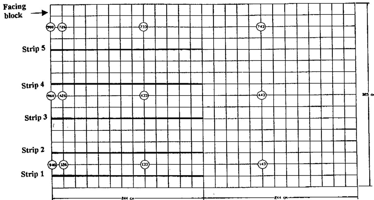
Figure 1. Finite element mesh of reinforced earth wall. Numbers in circle refer to nodes.
