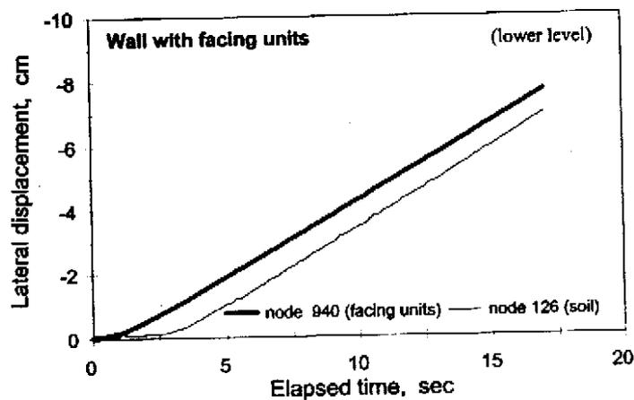
**Figure 6. Lateral displacement at lower level. Input acceleration in conjunction with surcharge 34 kPa**
