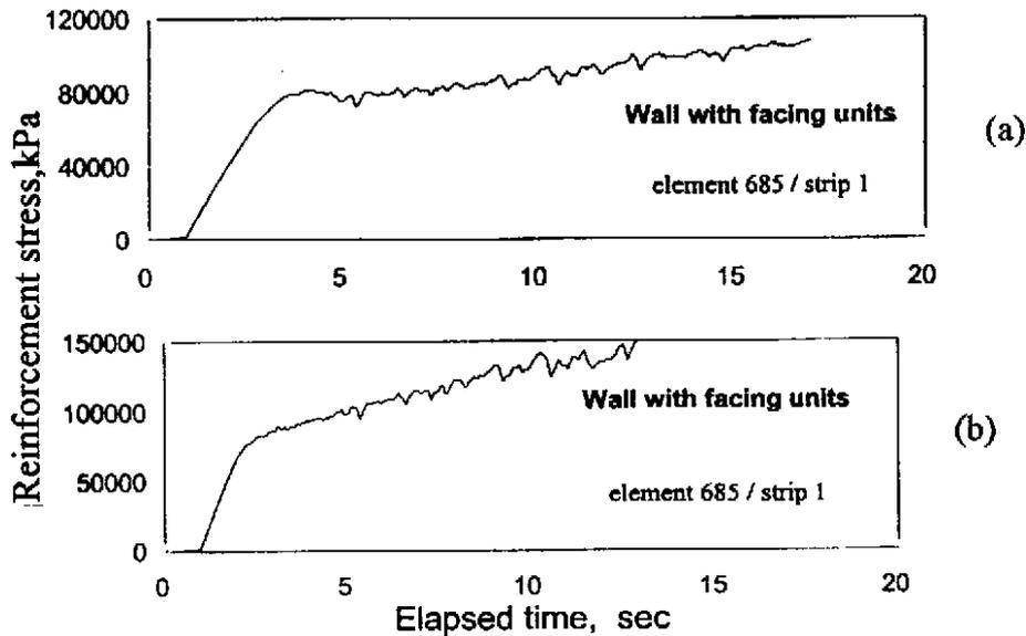
Figure 7. Tensile stress distribution in reinforcement. Input acceleration in conjunction with
