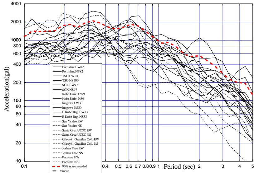
**Figure 2: Acceleration response spectra of observed records after compensated by attenuation relation using Equivalent Hypocentral Distance**
