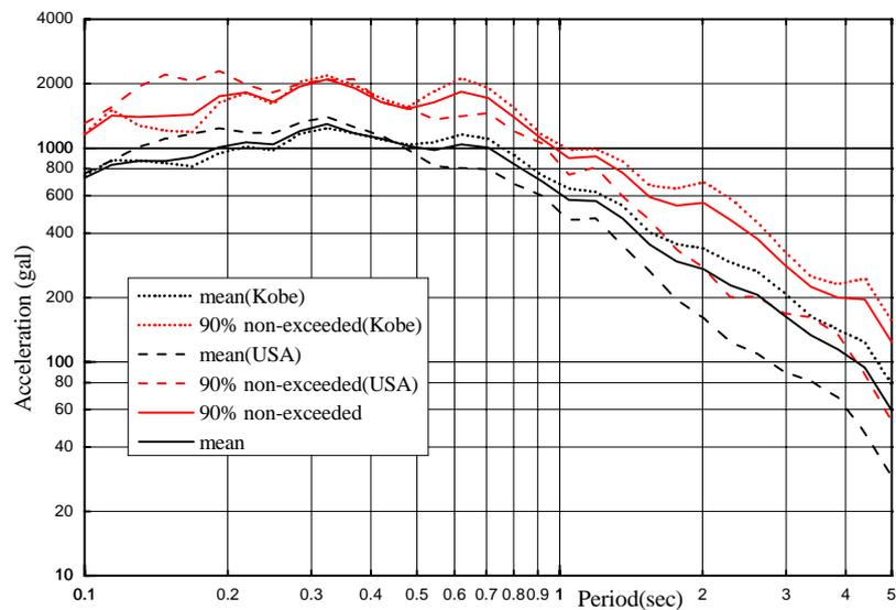
**Figure 3: Comparison of the statistical results based on the seismic records in USA and Kobe, respectively**
