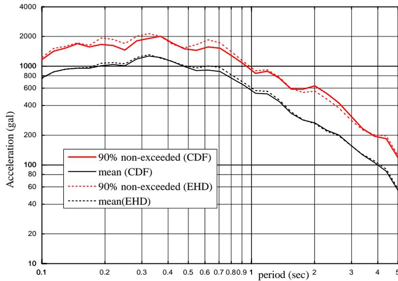
**Figure 4: Comparison of the statistical results using Closest Distance to Fault and Equivalent Hypocentral Distance attenuation relations**
