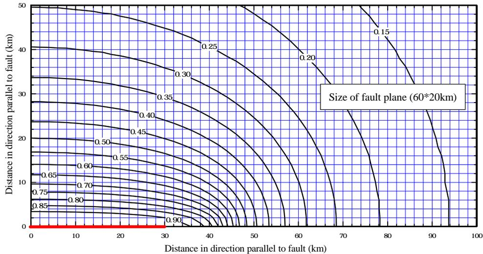
**Figure 6: Contour of reduction of ground motion near a fault**
