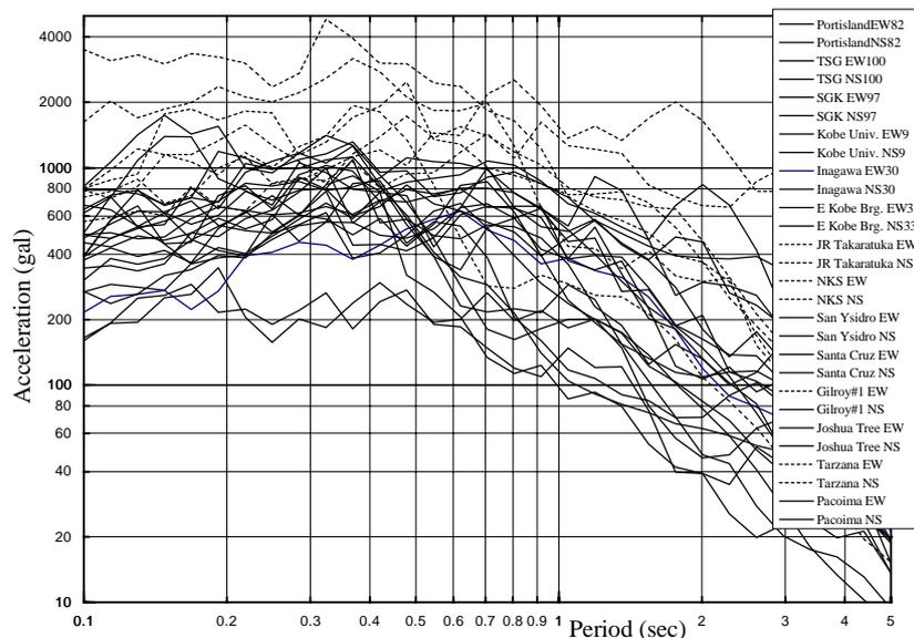
**Figure 1: Acceleration response spectra of observed records at near field area of inland earthquakes**
