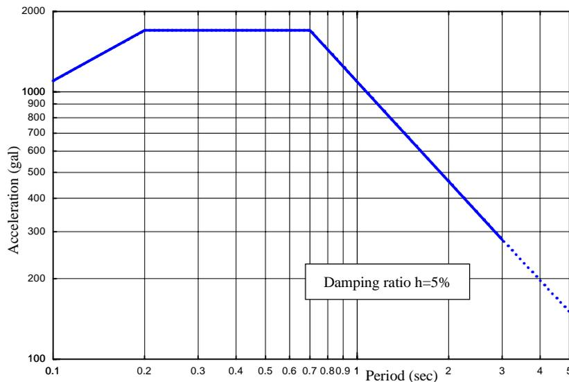
**Figure 5: Acceleration Response spectrum for design seismic motion straight above an inland fault**
