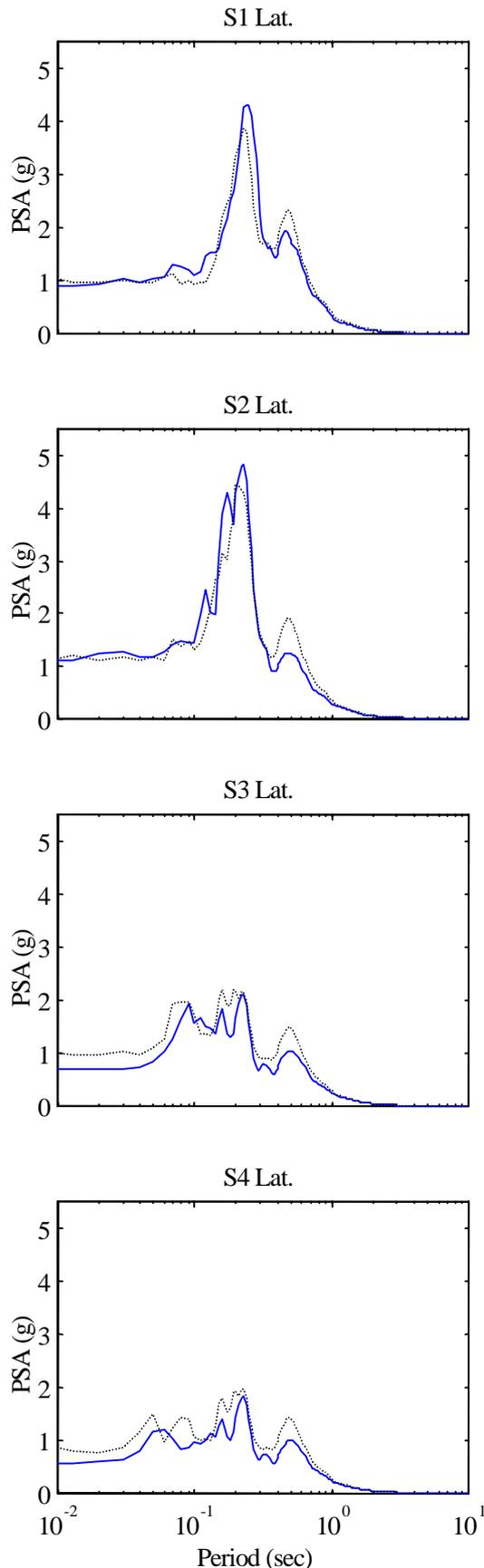
Figure 5: Comparison of Observed and Calculated Superstructure Response Spectra for Test 1.18
