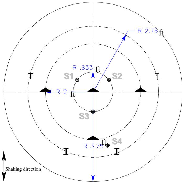
a) Plan View of Shaking Table Test 1.1
