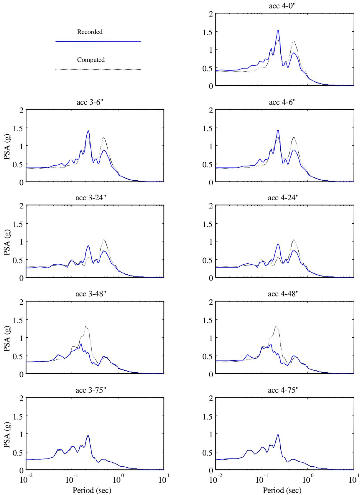
Figure 4: Comparison of Observed and Calculated Free Field Acceleration Response Spectra, Test 1.18.
