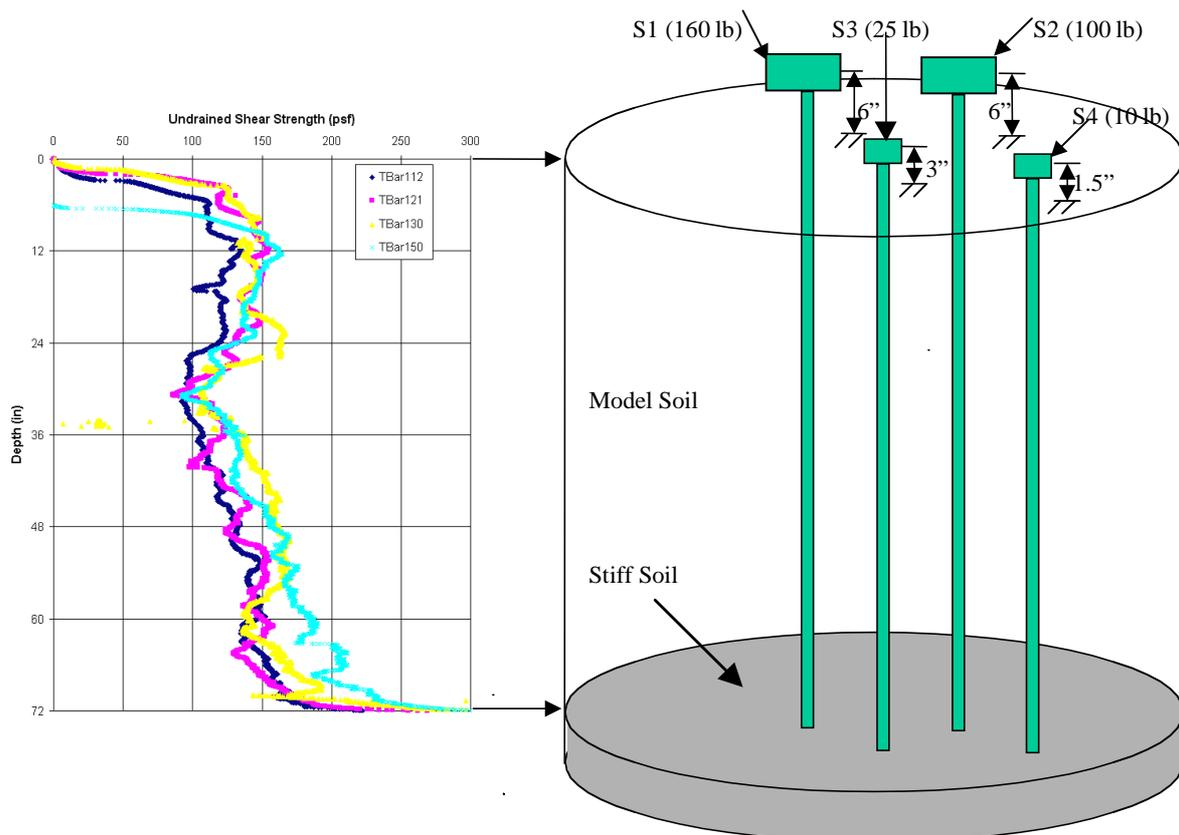
b) Shear Strength Profile and Set-up of Single Piles
