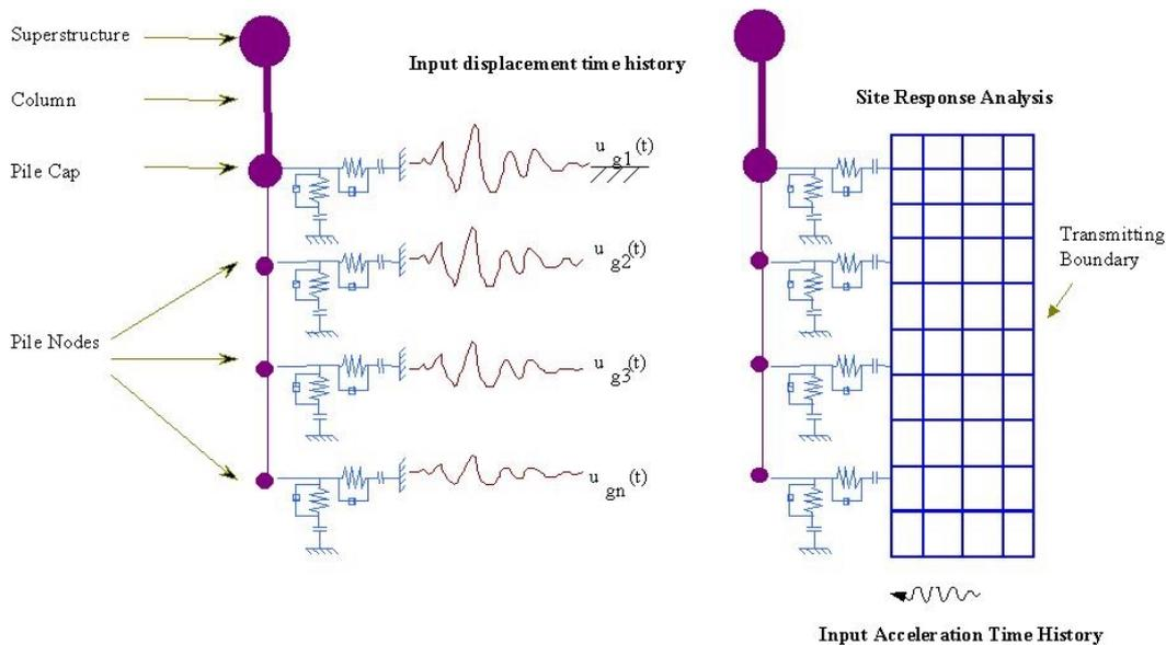
Figure 1: Uncoupled and Coupled Seismic Soil-Pile Interaction Diagram [modified from Abghari & Chai, 1995]
