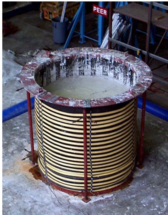
Figure 1. Model container on shaking table and filled with model soil
