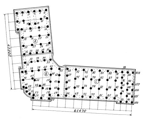
Figure 3. Layout of isolators
