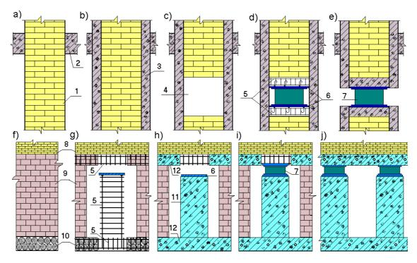
Figure 4. Remodeling of the isolators installation procedure
