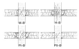
Figure 3: Cracking Pattern (Series B)
