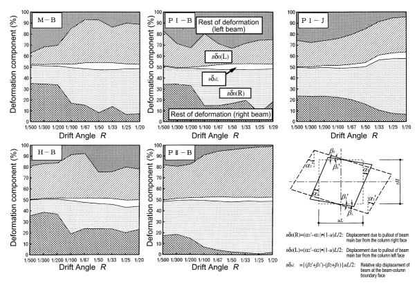
Figure 7: Deformation Component of Beam Member
