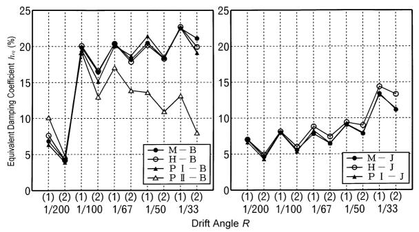
Figure 5: Comparison of Equivalent Damping Coefficient
