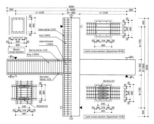
Figure 1: Details of Specimens
