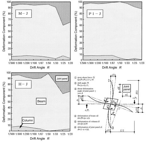
Figure 6: Deformation Component of Member (Series J)
