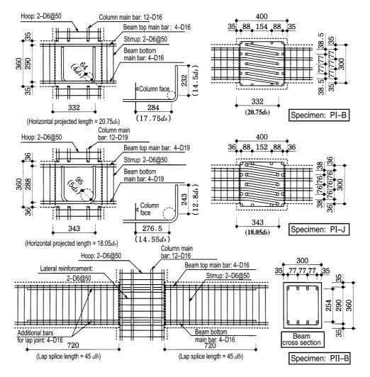
Figure 2: Details of Beam-Column Joints
