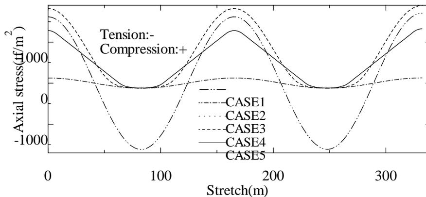
**Figure 6: Axial stress distribution of shield tunnel**
