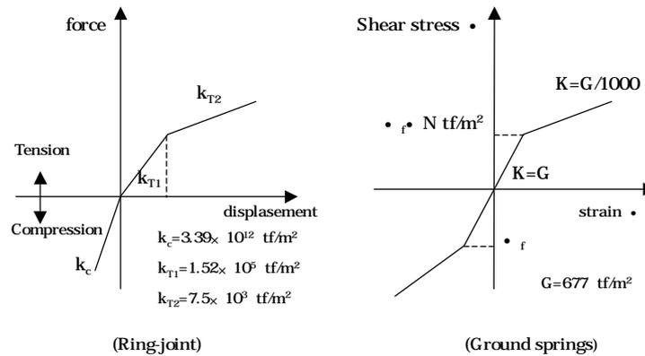
Figure 4: Non-linear features of the ring joints and the ground
