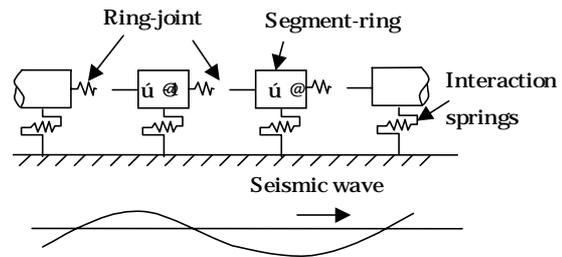
Figure 2: Model of Segment ring
