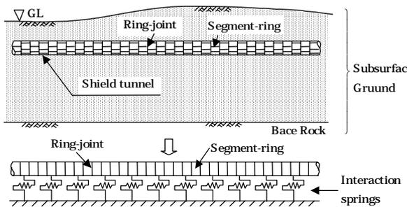
Figure 1: Modeling method for a shield tunnel
