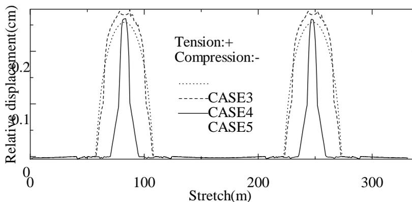
**Figure 8 : Relative displacement of ring joints**
