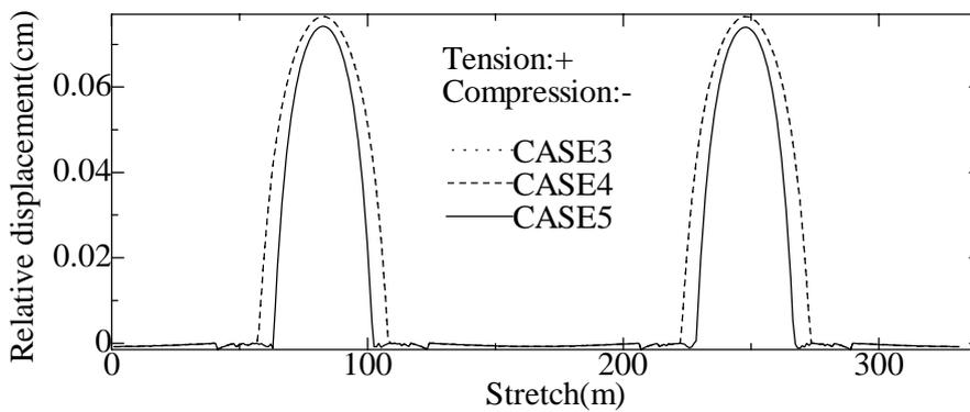
**Figure 5: Relative displacement of ring joint**
