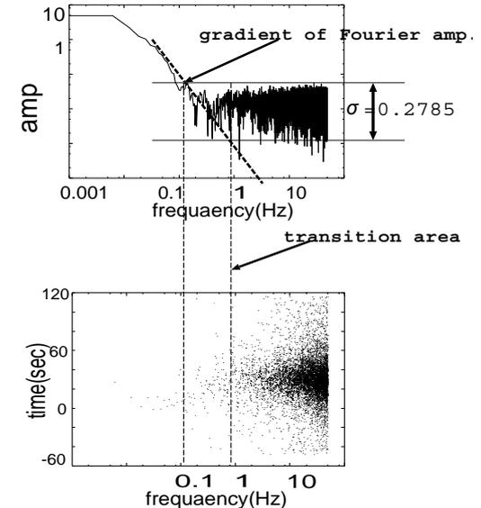
**Figure 6** Determination of transition area.
