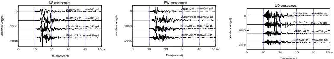
**Figure 2: Strong-motion records during the main-shock(NS, EW and UD components)**
