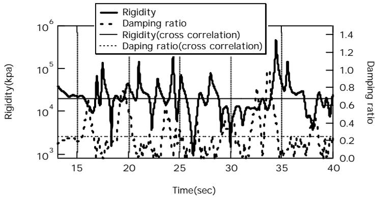
**Figure 8: Non-stationary variation of rigidity modulus and damping ratio estimated at 24 m depth**
