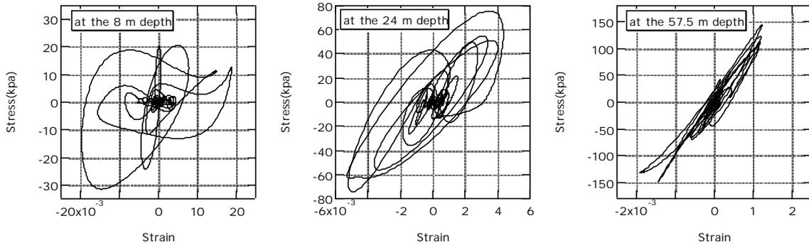
Figure 11: Stress and strain orbits at each depth
