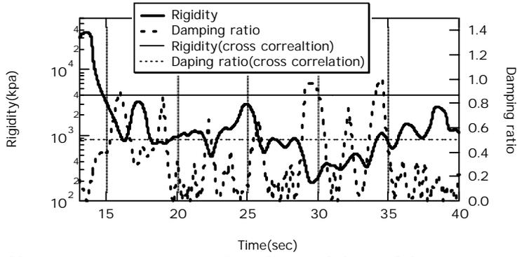
**Figure 7: Non-stationary variation of rigidity modulus and damping ratio estimated at 8 m depth**
