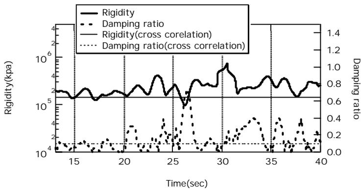
**Figure 9: Non-stationary variation of rigidity modulus and damping ratio estimated at 57.5 m depth**
