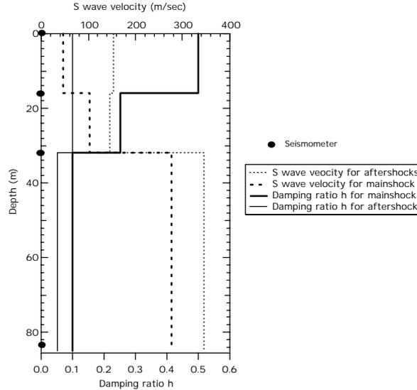
**Figure 6: Damping ratios estimated from the spectral fitness method with the reproduced velocities**
