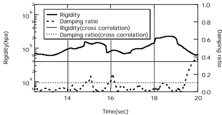
Figure 14: Rigidity modulus and damping ratio estimated at 24 m depth for an after-shock
