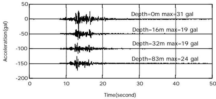
Figure 12: Strong-motion records during an after-shock (EW component)
