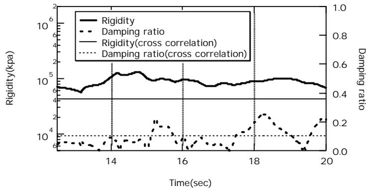
Figure 13: Rigidity modulus and damping ratio estimated at 8 m depth for an after-shock
