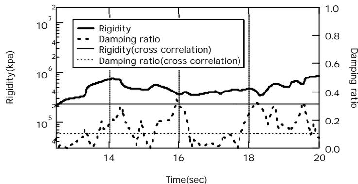
**Figure 15: Rigidity modulus and damping ratio estimated at 57.5 m depth for an after-shock**
