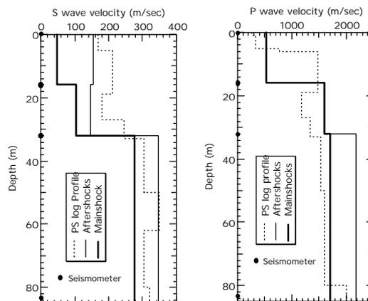
**Figure 5: S and P waves' velocities estimated from the cross correlation analyses**
