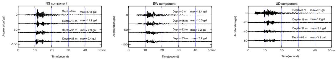
**Figure 3: Strong-motion records during an after-shock (NS, EW and UD components)**
