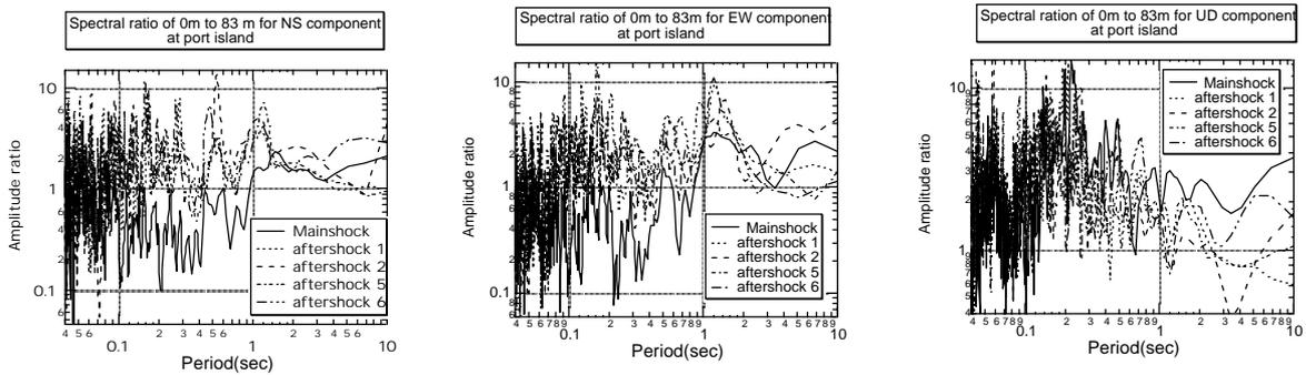
**Figure 4: Spectral ratios of the 0 m records to 83 m records (NS, EW and UD components)**
